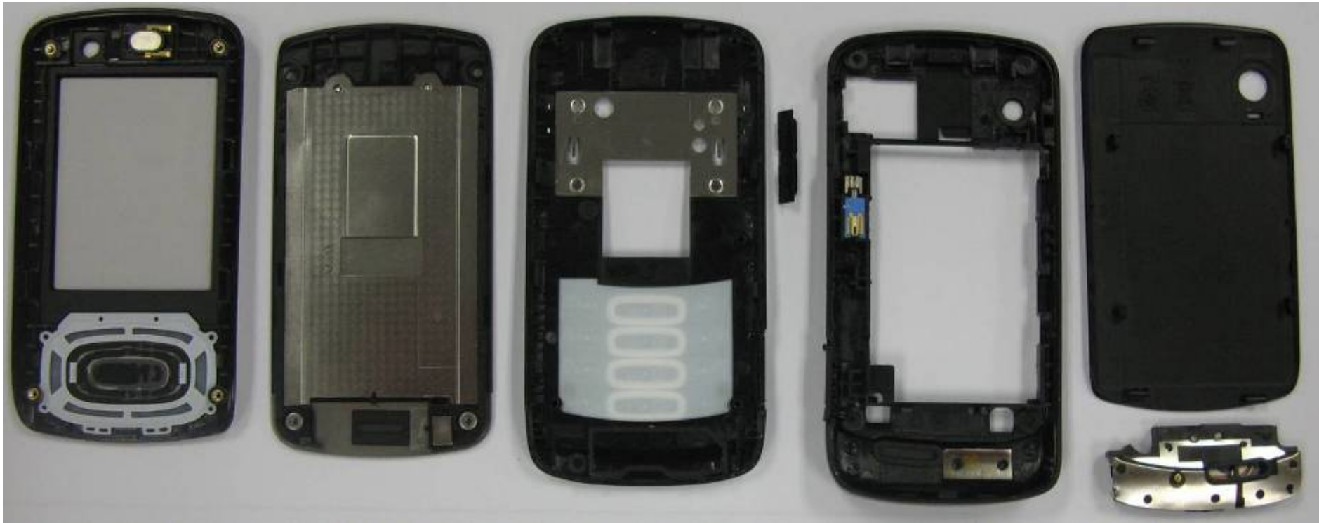
Internal View of housings
