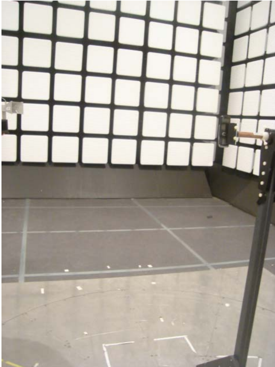
22718-1, IHDT56KP2 setup in semi-anechoic chamber – right view (18 GHz – 26.5 GHz)
