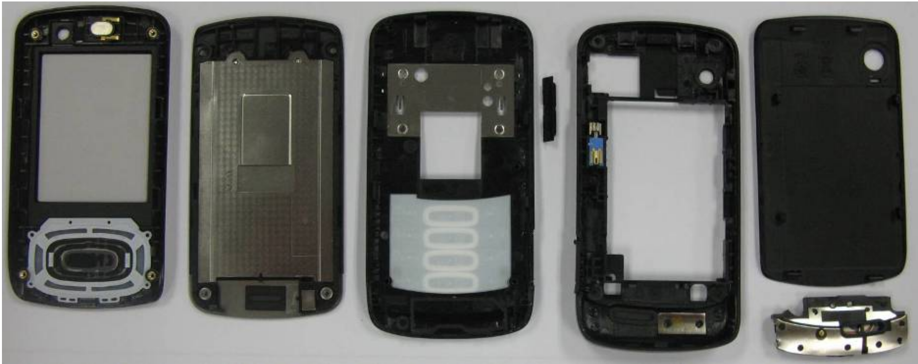
Internal View of housings
