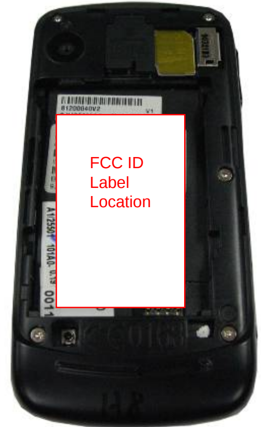
Rear View with Battery Cover Removed
