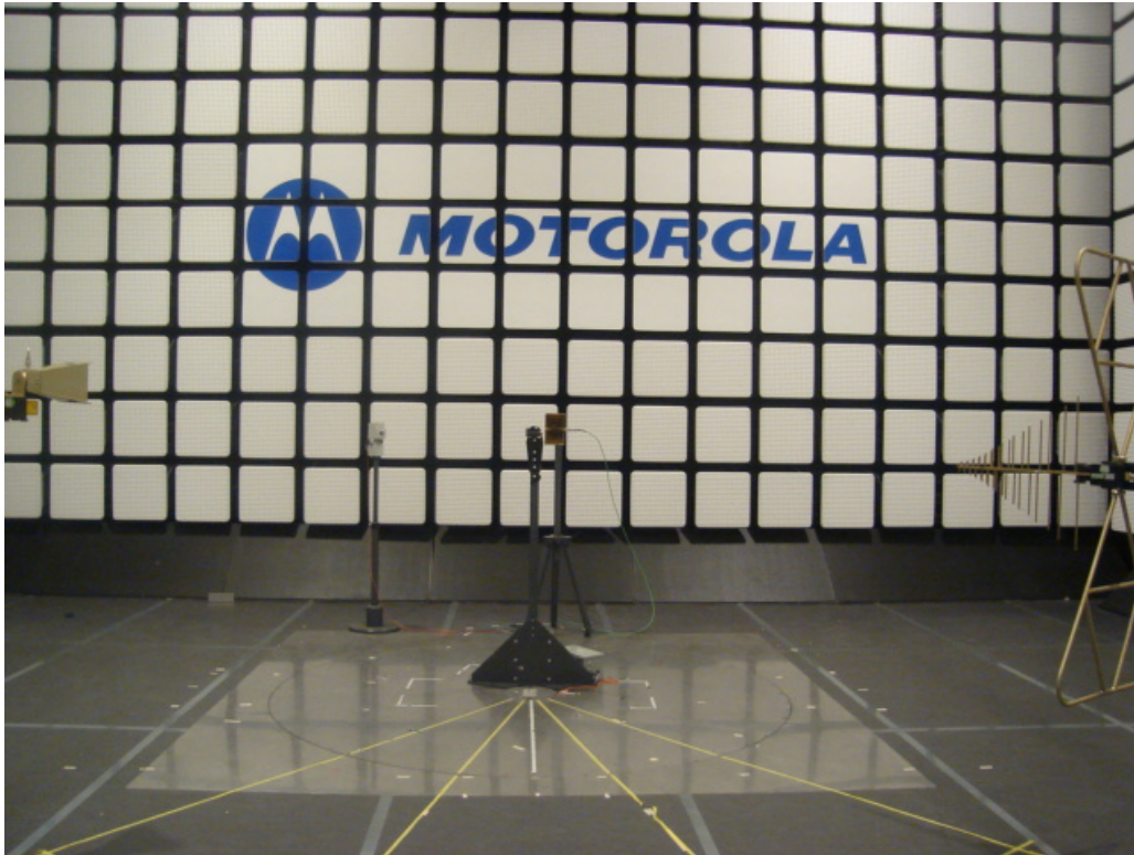
22874-1, IHDT56KP1 setup in semi-anechoic chamber – front view (30 MHz – 18 GHz)
