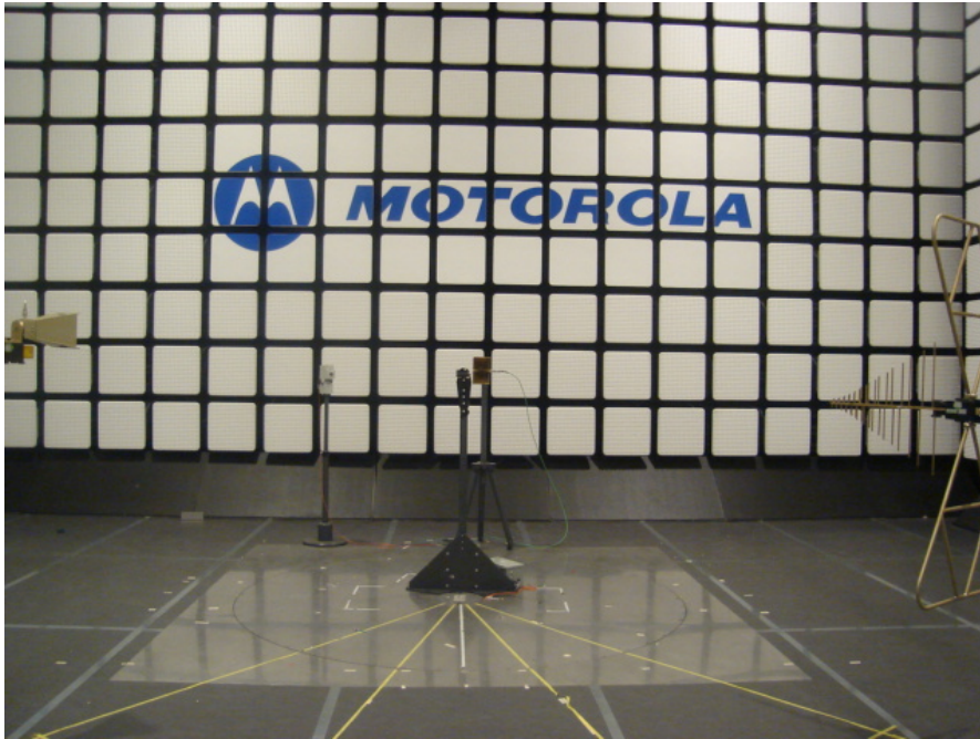
22826-1, IHDT56KJ1 setup in semi-anechoic chamber – front view (30 MHz – 18 GHz)
