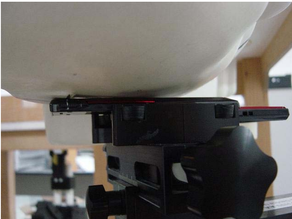
Figure 6: Phone against the Head Phantom (Cheek Touch – Slide Open)
