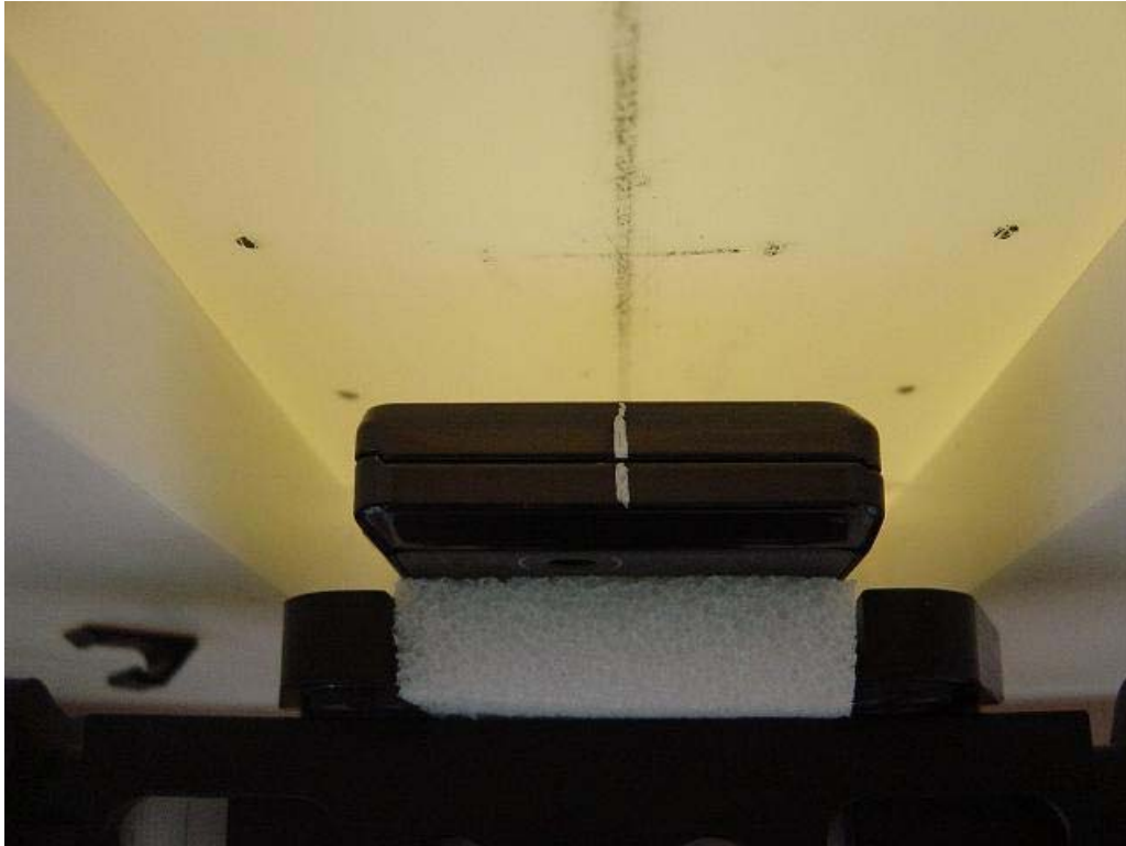
Figure 9: Phone against the Flat Phantom
