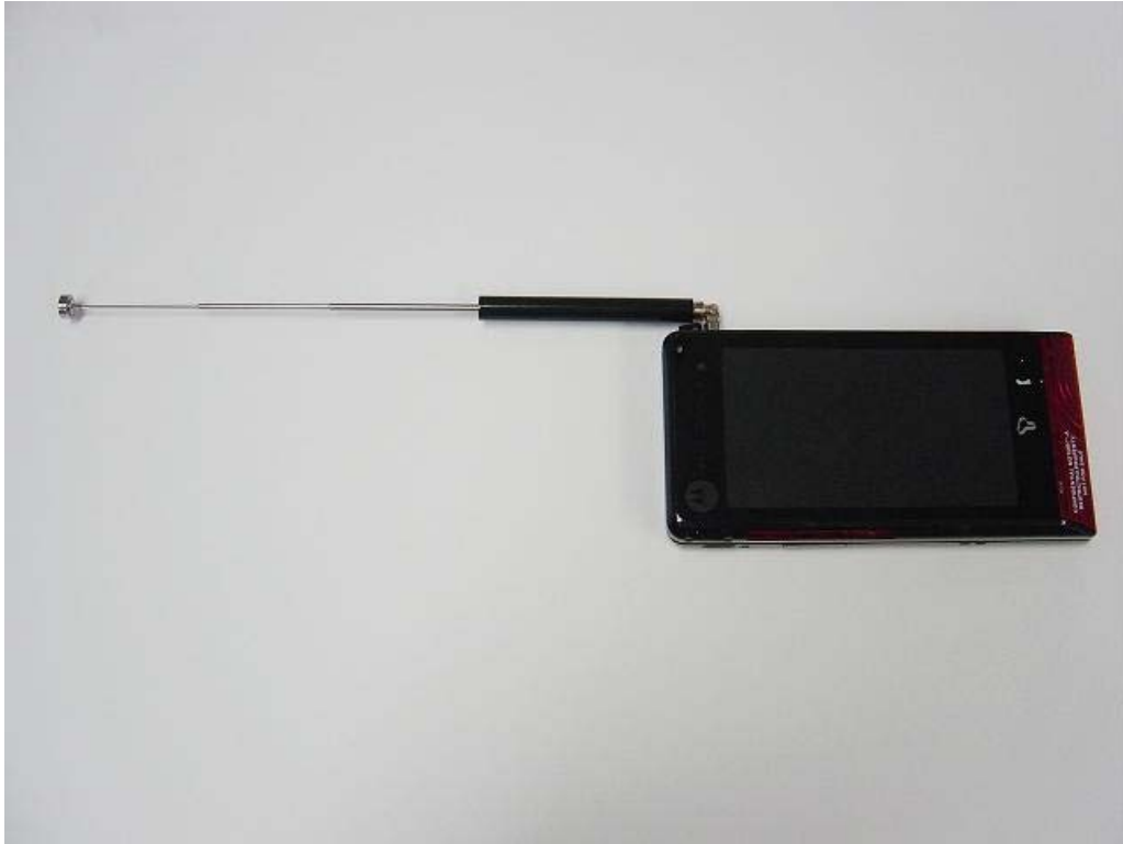
Figure 11: Phone with DMB Antenna of Position 1 extended
