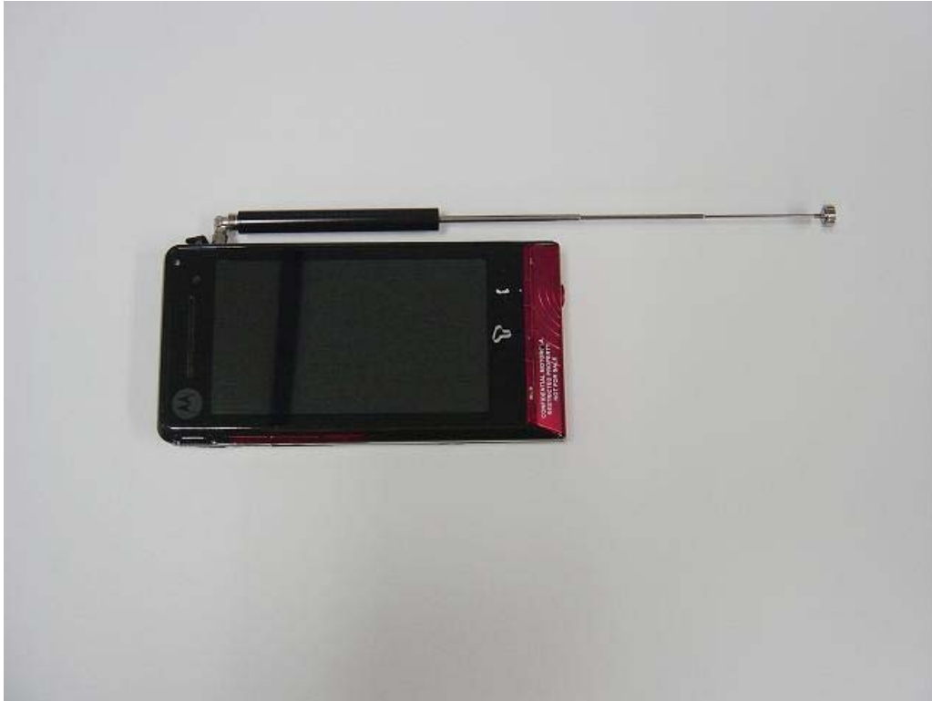
Figure 13: Phone with DMB Antenna of Position 2 extended
