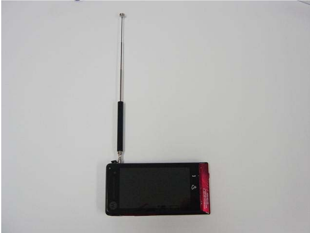
Figure 15: Phone with DMB Antenna of Position 3 extended
