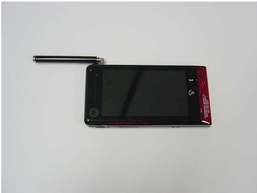
Figure 10: Phone with DMB Antenna of Position 1 retracted
