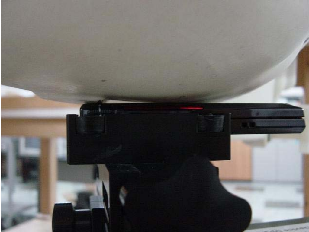
Figure 5: Phone against the Head Phantom (Cheek Touch – Slide Close)
