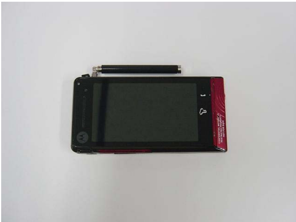
Figure 12: Phone with DMB Antenna of Position 2 retracted
