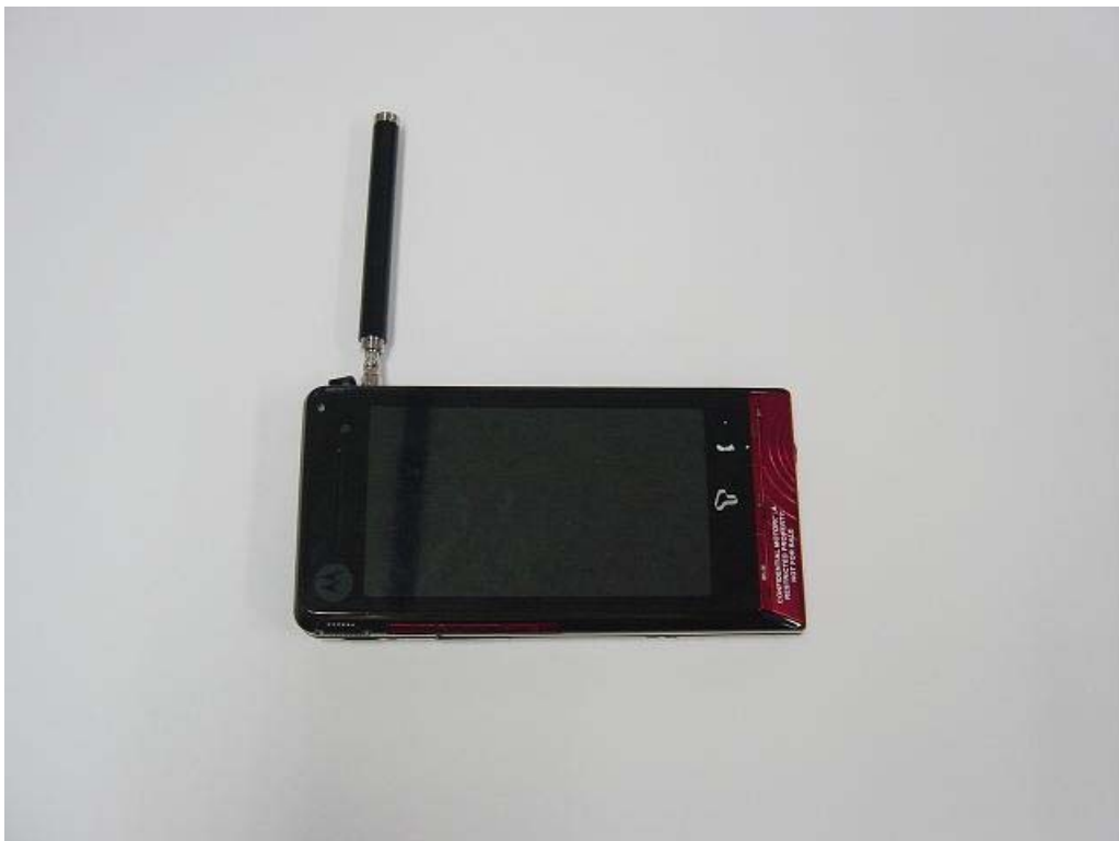
Figure 14: Phone with DMB Antenna of Position 3 retracted
