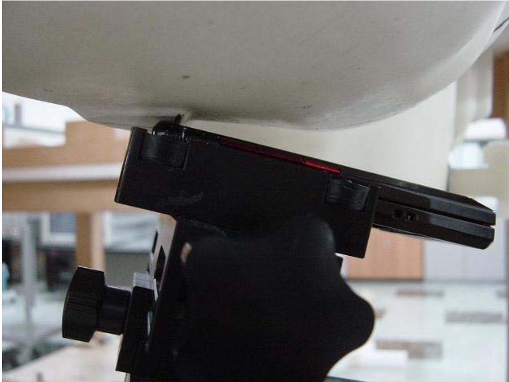
Figure 7: Phone against the Head Phantom (15° Tilt – Slide Close)
