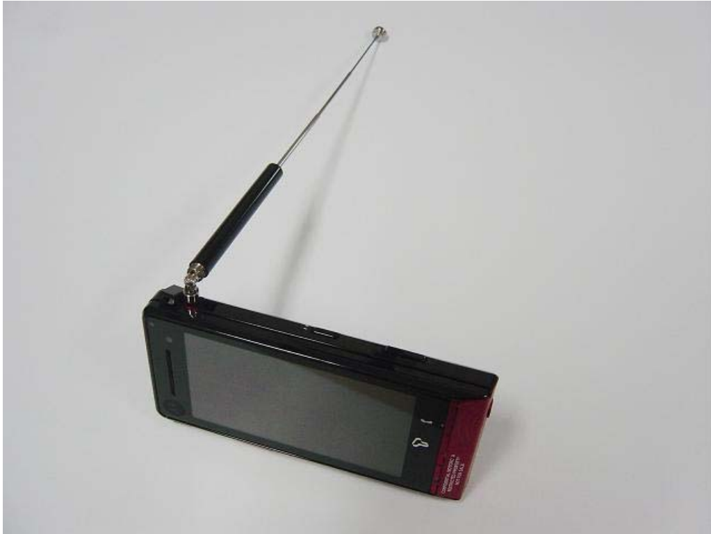
Figure 17: Phone with DMB Antenna of Position 4 extended
