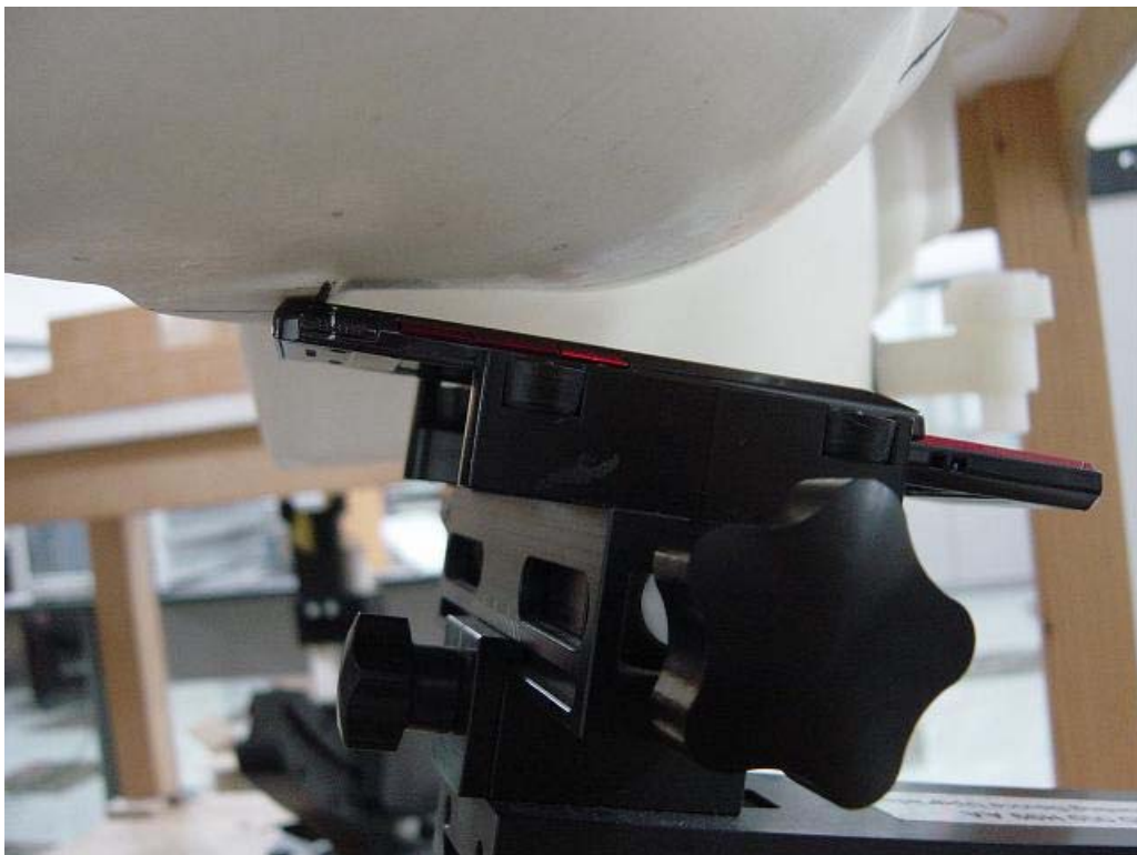
Figure 8: Phone against the Head Phantom (15° Tilt – Slide Open)
