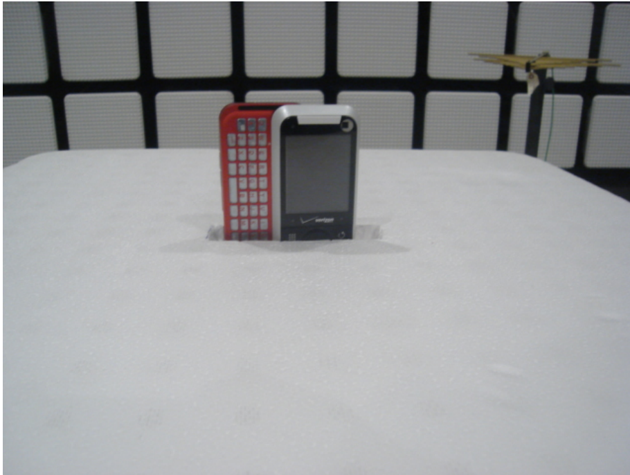
22631-1, IHDT56KG1 placed in test position Z – Slider open
