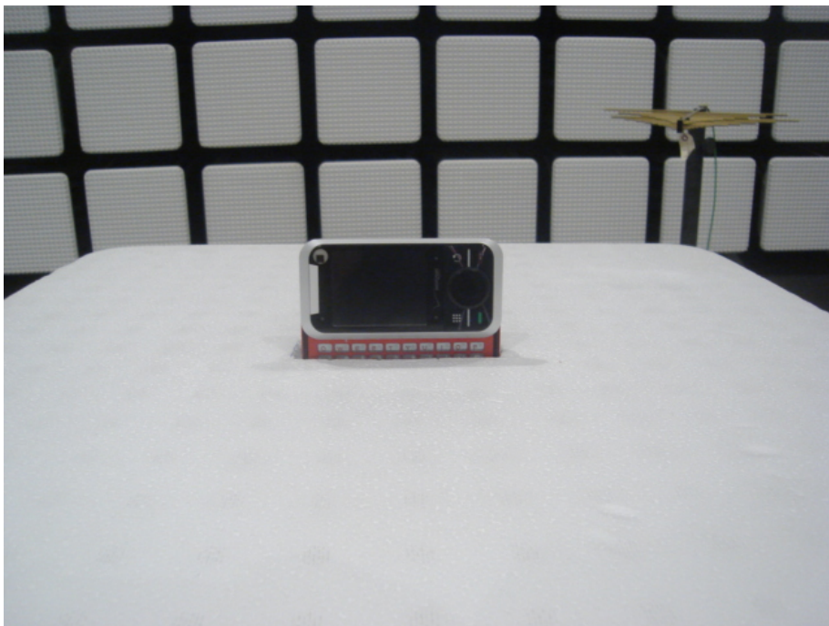
22631-1, IHDT56KG1 placed in test position Y – Slider open
