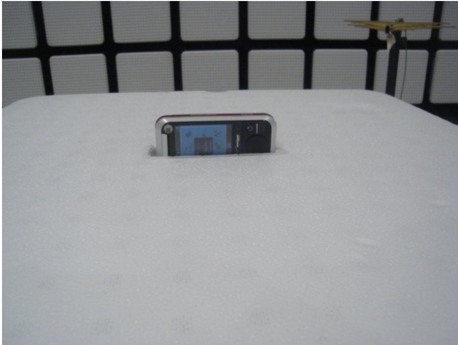
22631-1, IHDT56KG1 placed in test position Y – Slider closed
