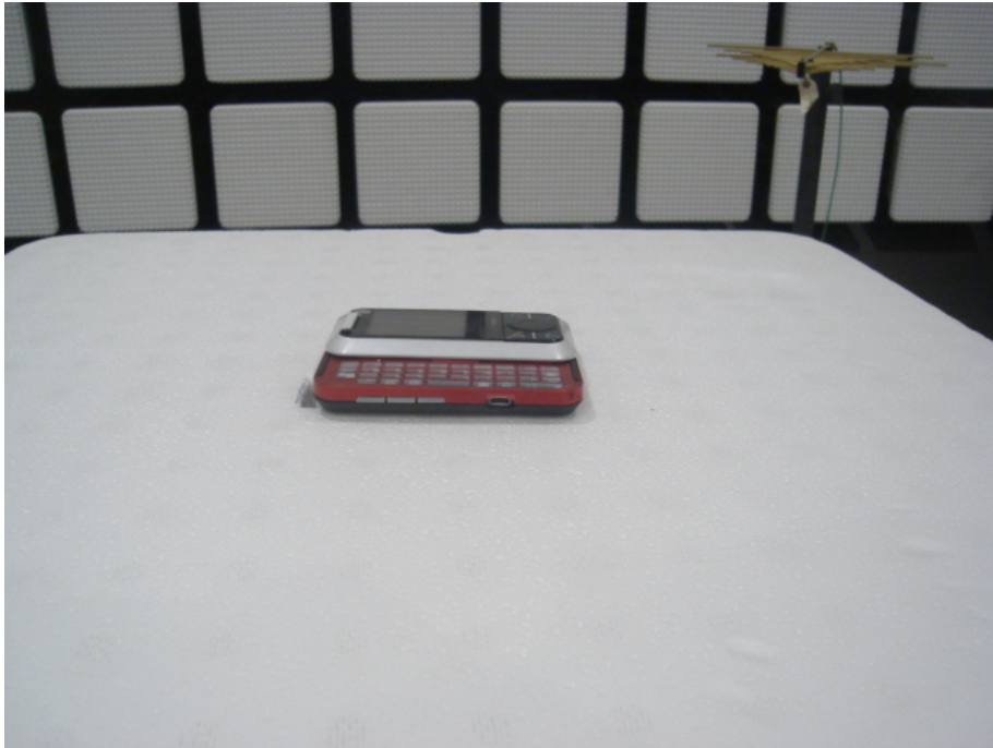
22631-1, IHDT56KG1 placed in test position X – Slider open
