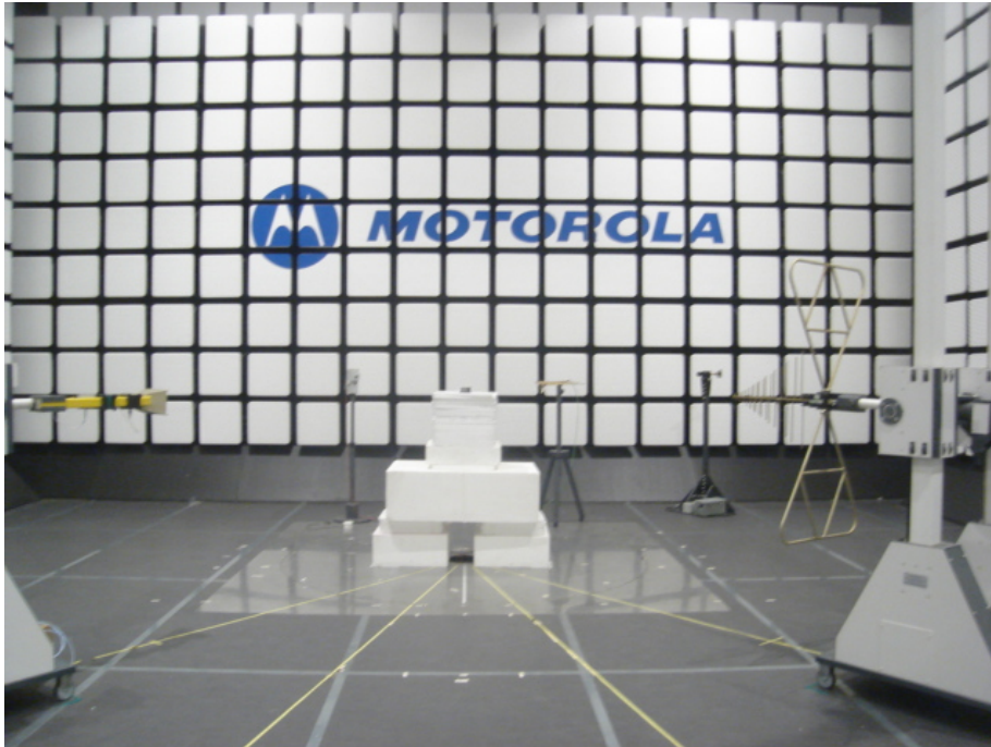
22631-1, IHDT56KG1 setup in semi-anechoic chamber – front view (30 MHz-18 GHz)
