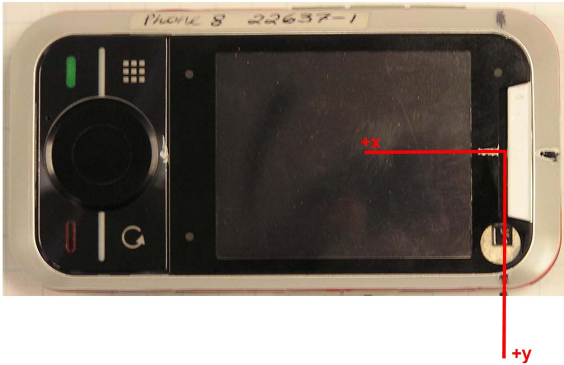
Figure 5. Coordinate Axis for Telecoil Measurements
