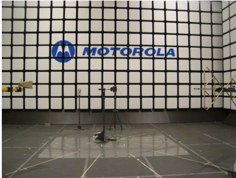
22708-1, IHDT56KE1 setup in semi-anechoic chamber – front view (30 MHz – 18 GHz)
