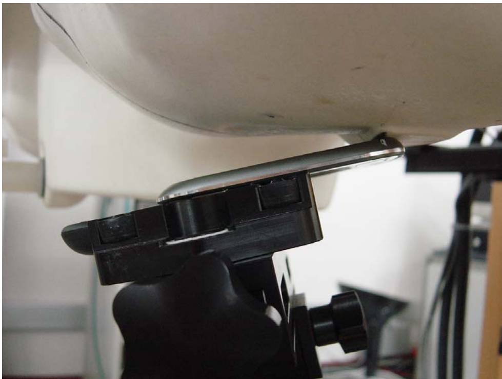
Figure 8: Phone Against the Head Phantom (15° Tilt – Slider Up)
