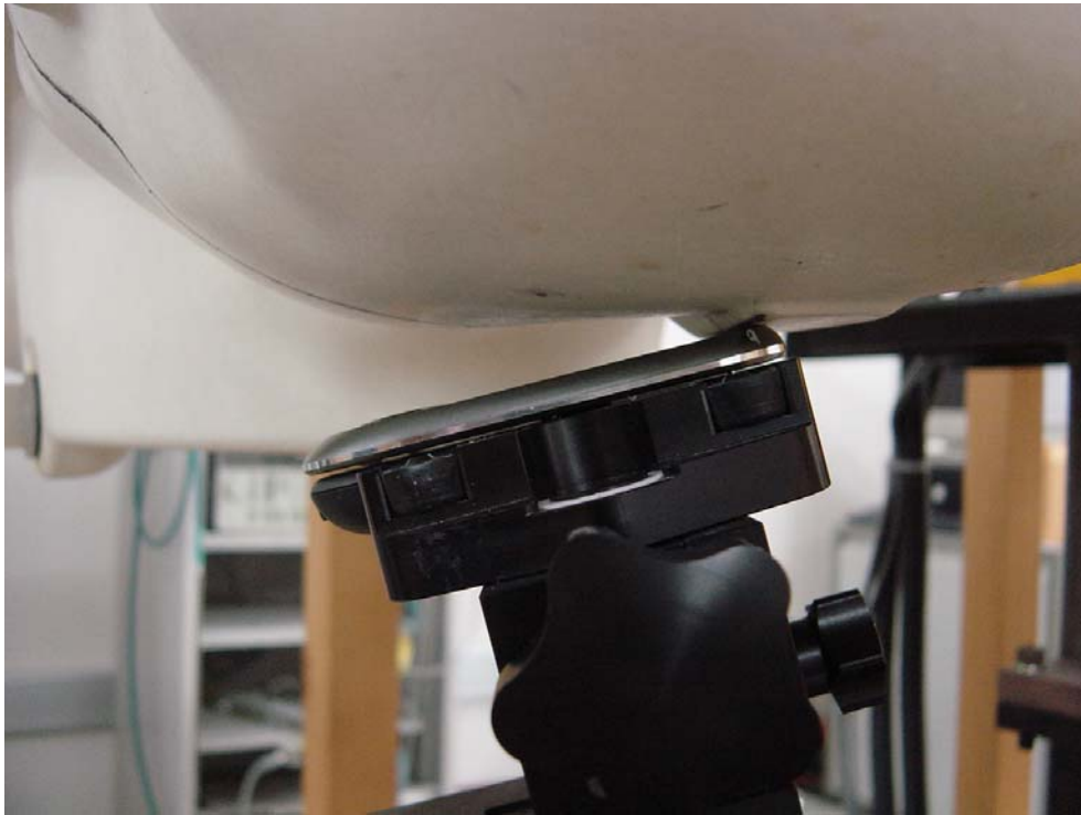
Figure 7: Phone Against the Head Phantom (15° Tilt – Slider Down)
