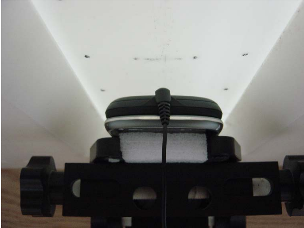
Figure 9: Phone Against the Flat Phantom
