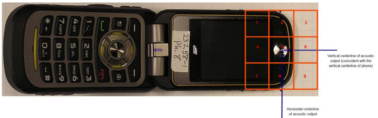
Figure 2. Phone Front - Orientation and Measurement Plane for RF Emissions Testing
