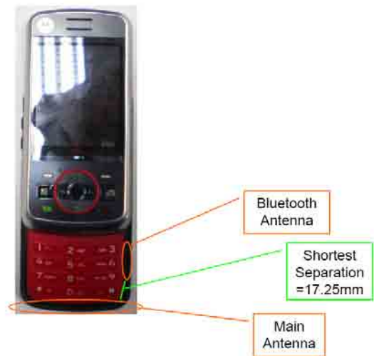
Banfi Antenna Separation
