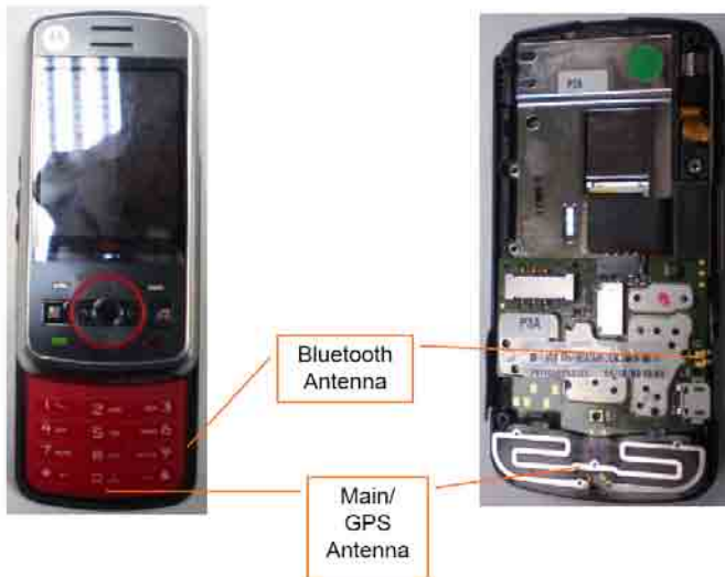
Banfi Internal Antenna Locations
