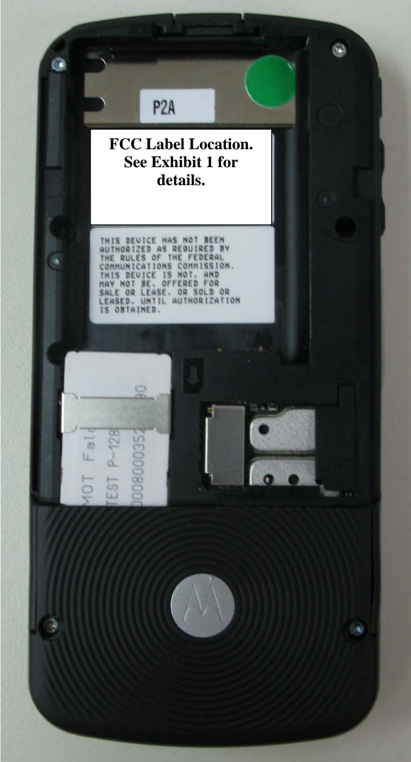
Figure 3-9. Interior Compartment of radio
