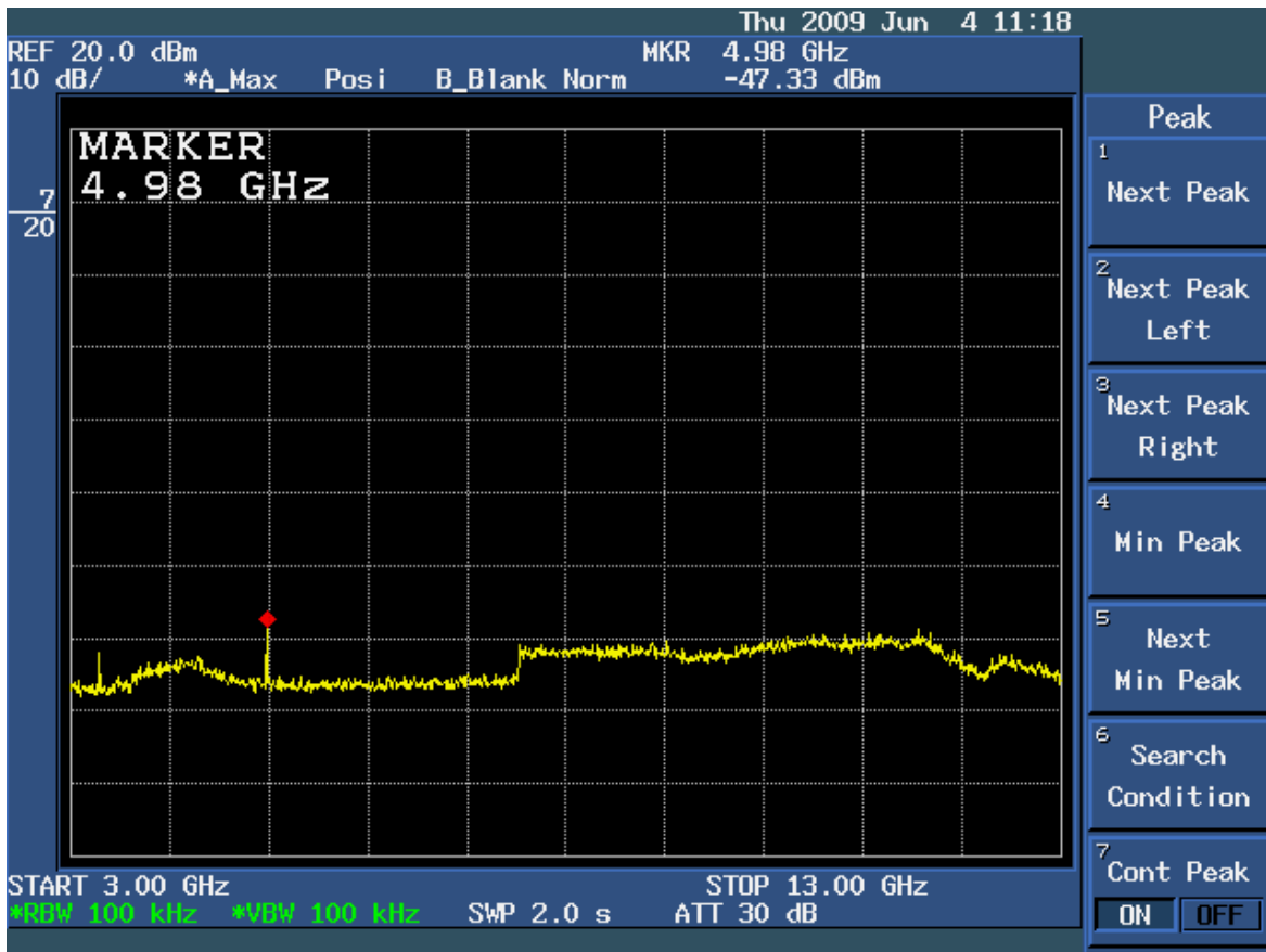
Figure 6c.7-8: Plot of spurious conducted emissions 3 GHz – 13 GHz (High Channel Enabled).
