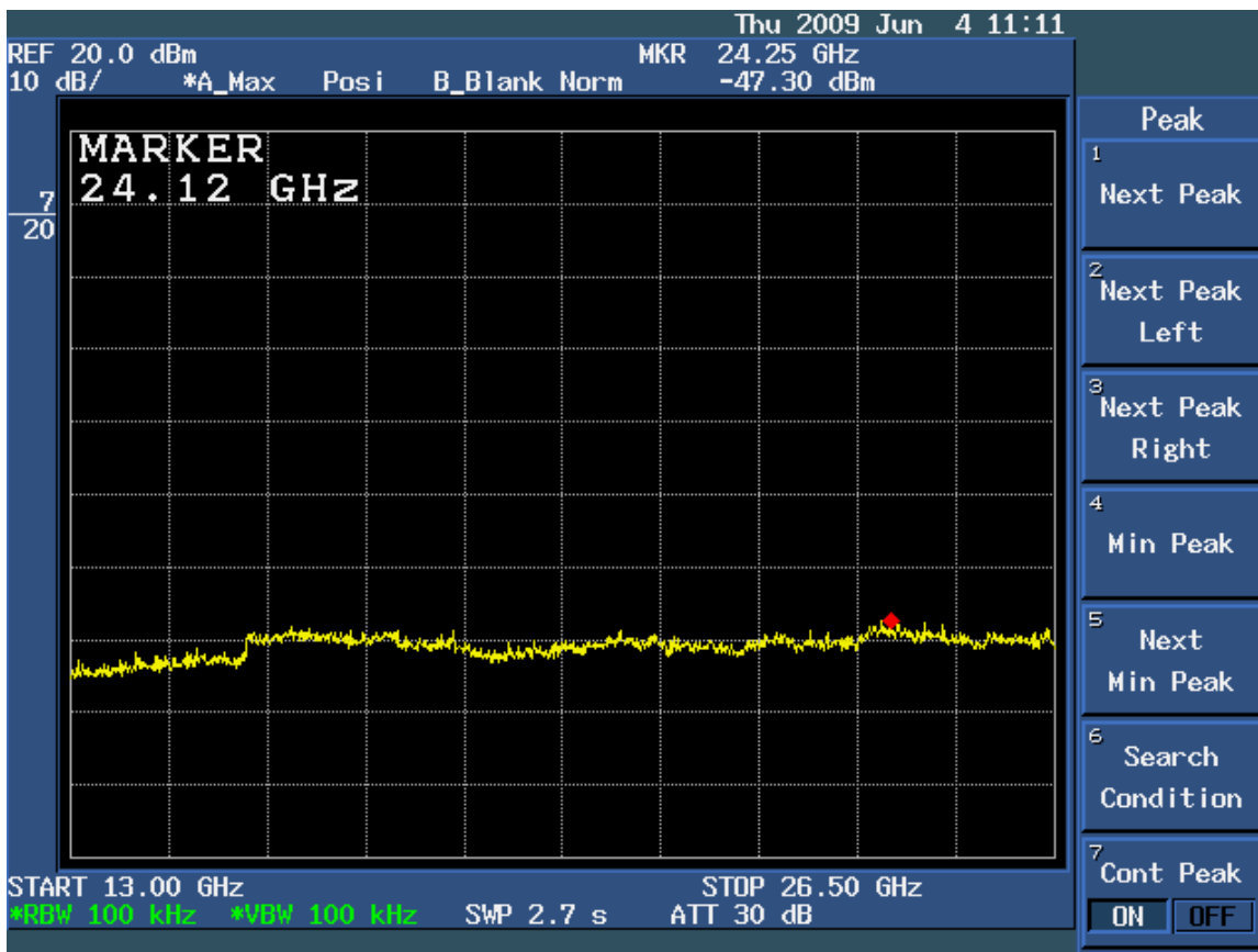
Figure 6c.7-3: Plot of spurious conducted emissions 13 GHz – 26.5 GHz (Low Channel Enabled).
