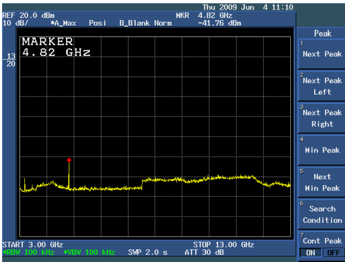
Figure 6c.7-2: Plot of spurious conducted emissions 3 GHz – 13 GHz (Low Channel Enabled).
