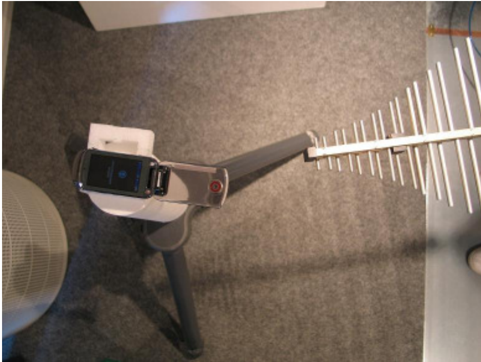
21841-1, IHDT56JZ1 Check for maximum radiation at position X - Open
