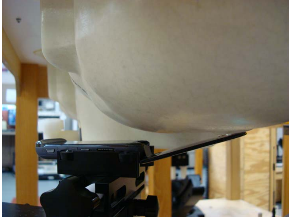
Figure 5 – Transceiver against head, 15° Tilt position
