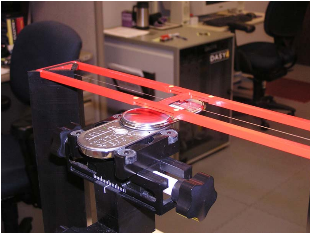
Figure 4. Positioning and Measurement for RF Emissions
