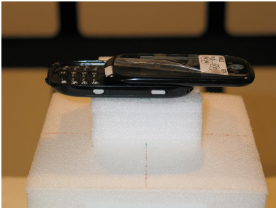
22089-1, IHDT56JW1 placed in test position X - Open
