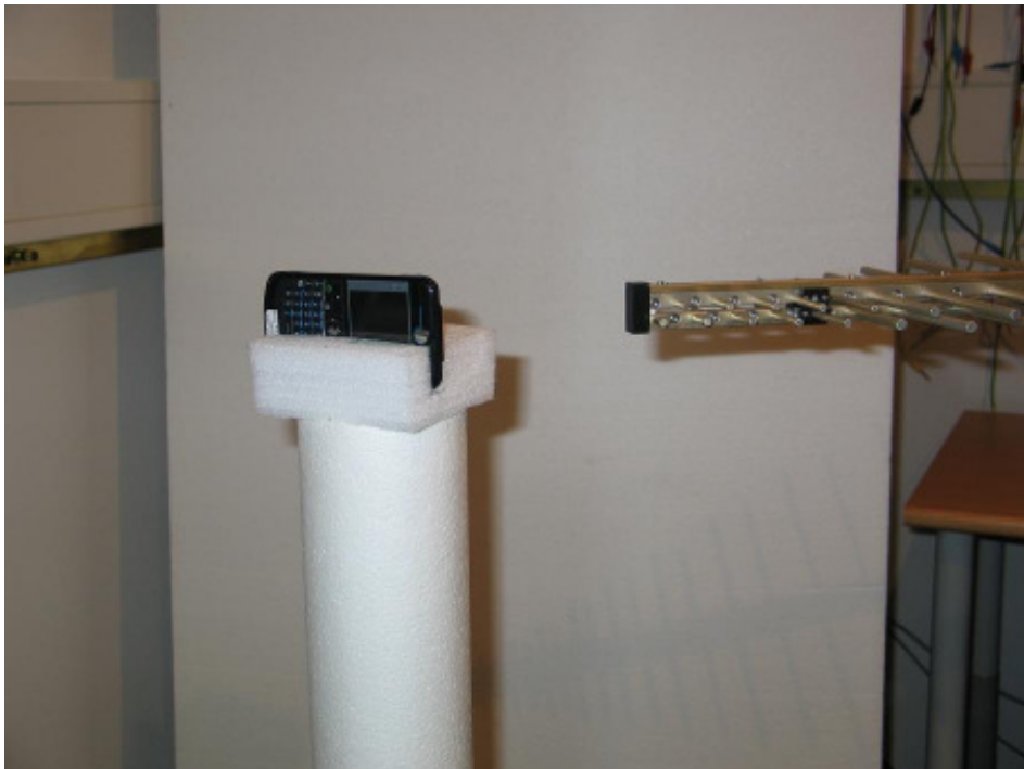
21897-2, IHDT56JV1 Check for maximum radiation at position Y – BT/WiFi band (g) mode
