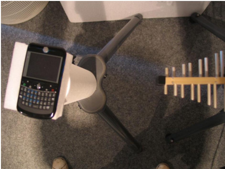
21897-2, IHDT56JV1 Check for maximum radiation at position X – WiFi band (b) mode
