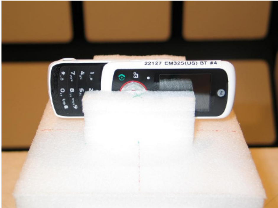
22127-1, IHDT56JU1 placed in test position Y – Open
