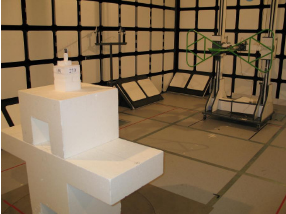
22127-1, IHDT56JU1 setup in semi-anechoic chamber – left side
