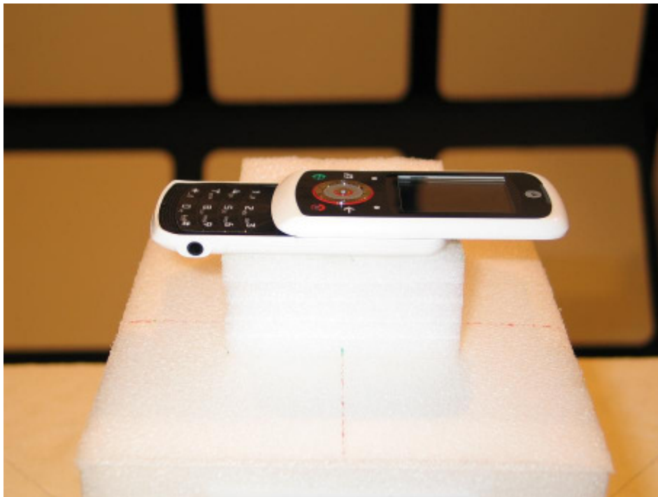
22127-1, IHDT56JU1 placed in test position X – Open
