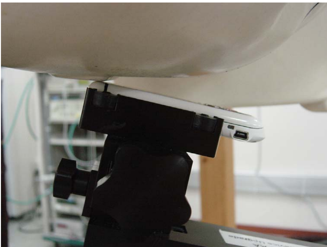
Figure 6: Phone Against Head Phantom (15° Tilt)
