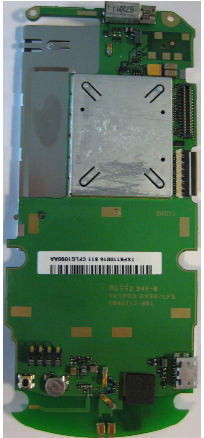
BACK SIDE OF MAIN PCB WHERE YOU CAN SEE THE BACK OF THE DISPLAY DB REMOVED
