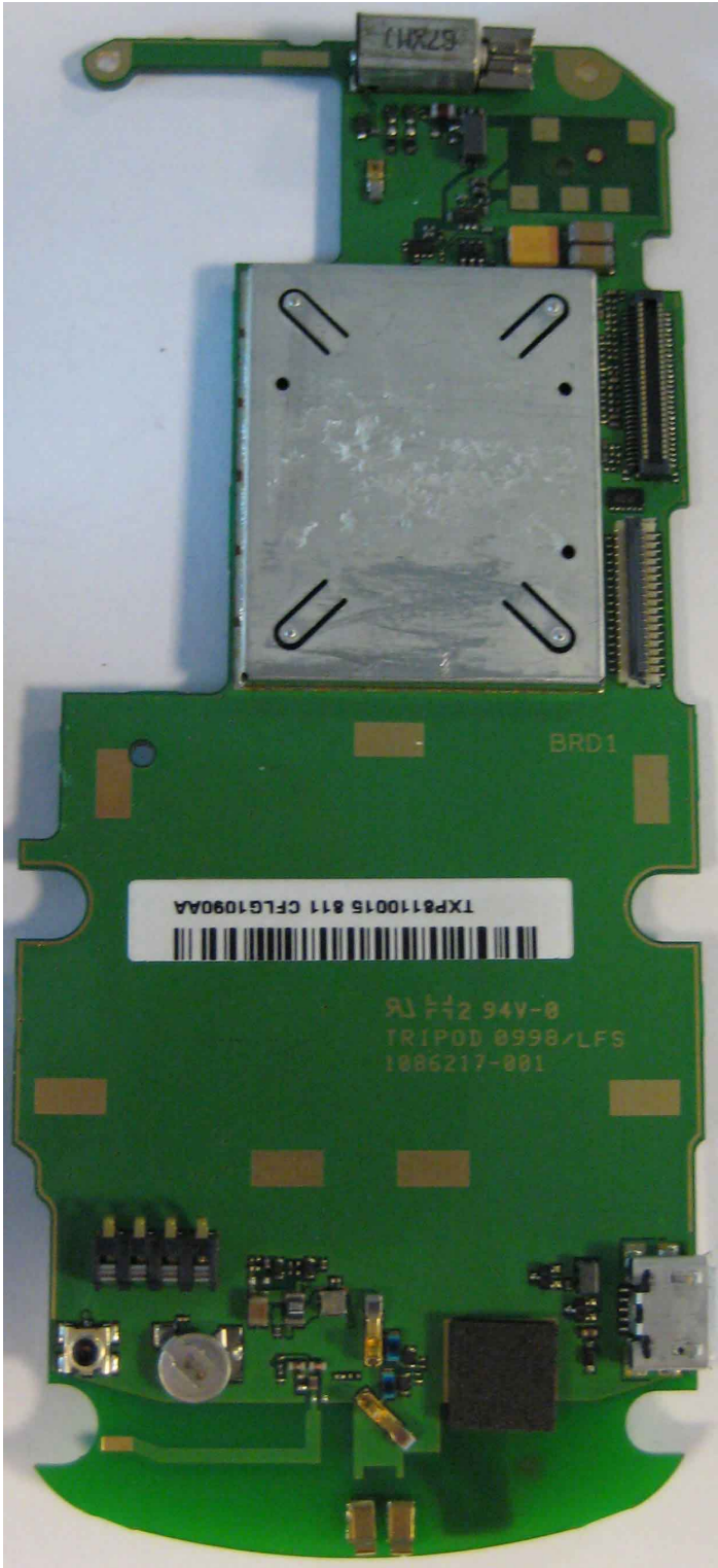
MAIN PCB WITH SHIELD
