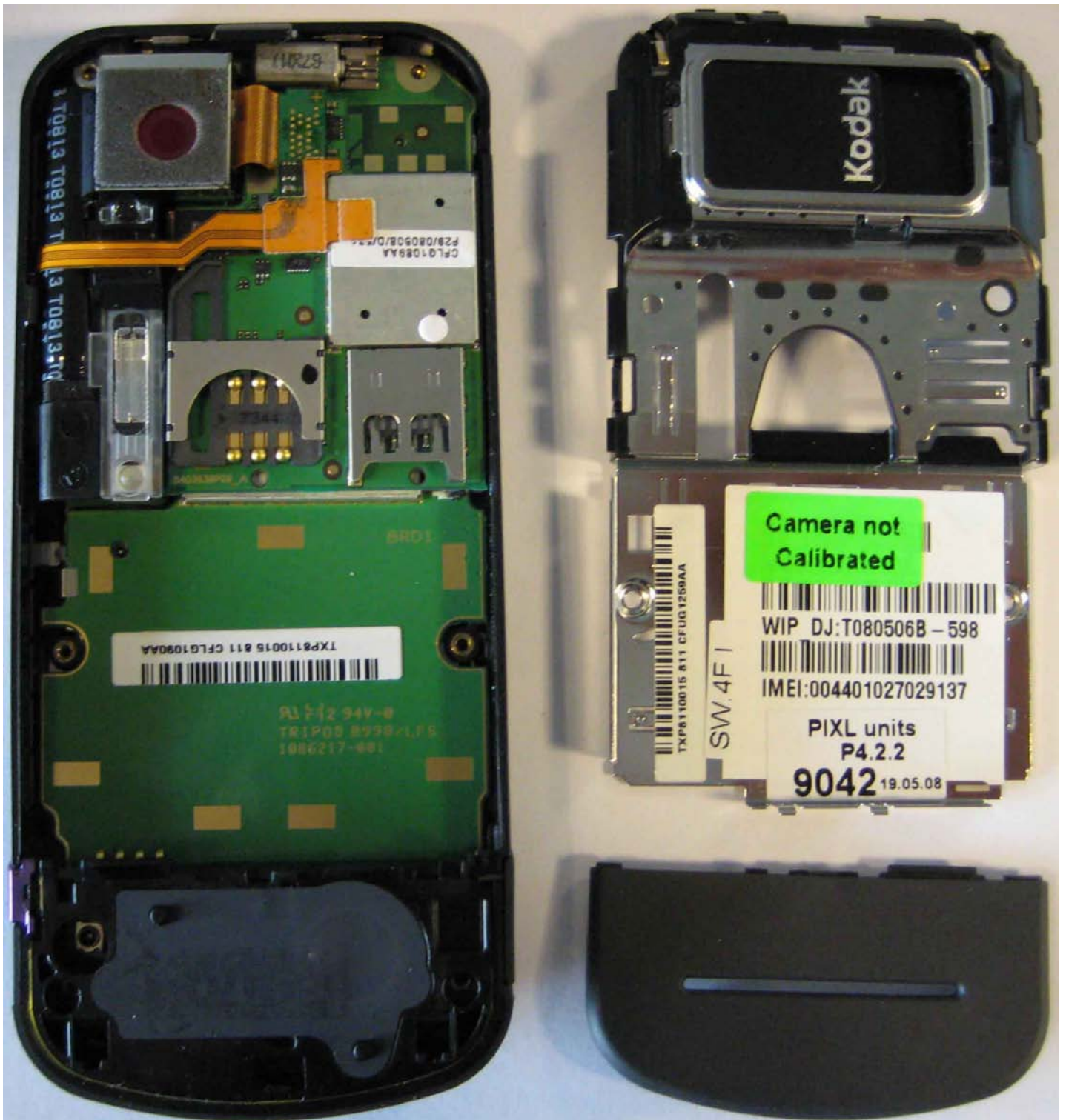
REAR PART REMOVED FROM PHONE
