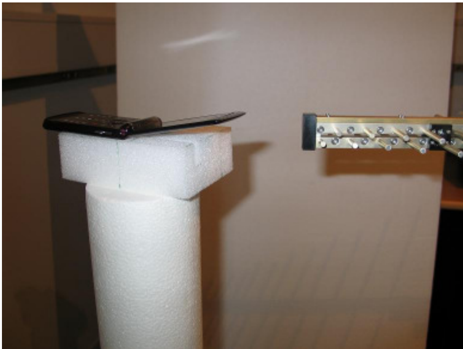
21832-1, IHDT56JR1 Maximum radiation position X - Open
