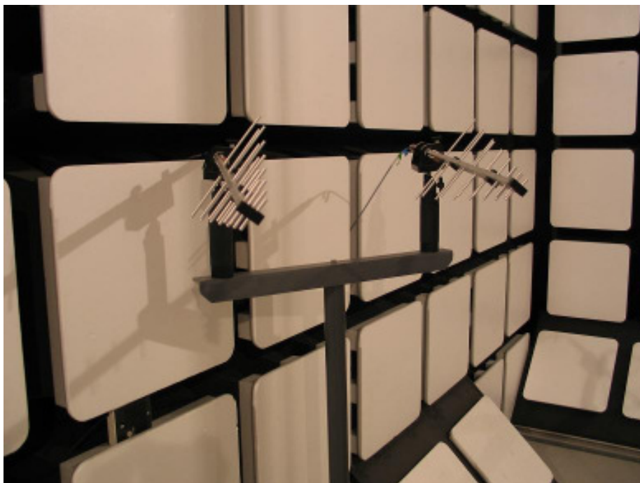
21832-1, IHDT56JR1 Orientation of link antennas
