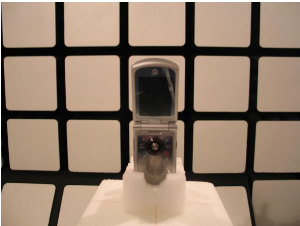
21616-1, IHDT56JM1 placed in test position Z - Open
