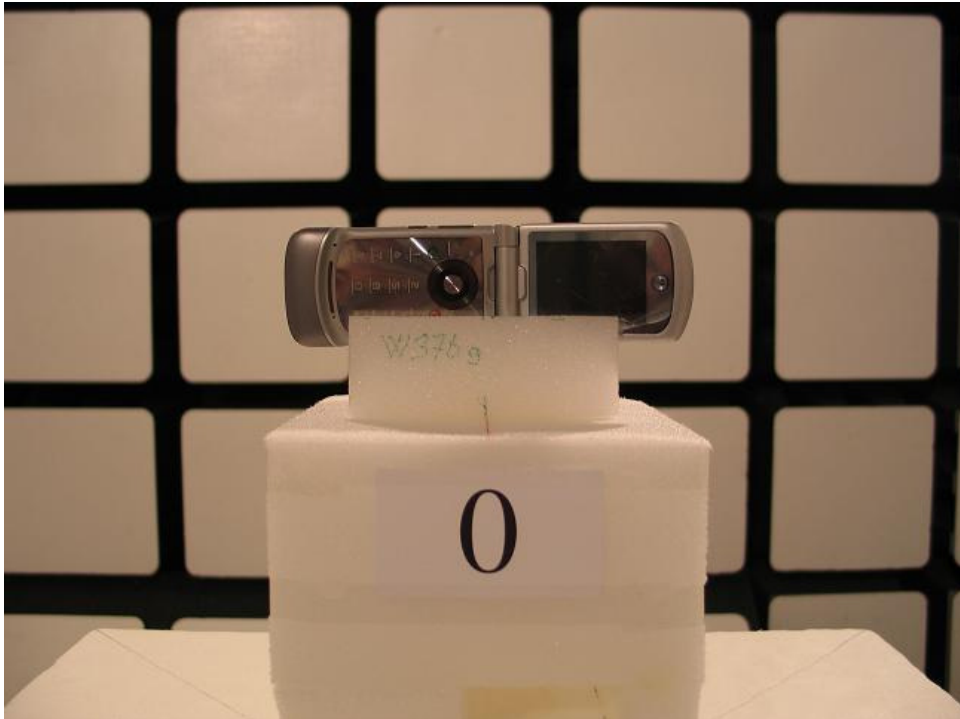
21616-1, IHDT56JM1 placed in test position Y - Open
