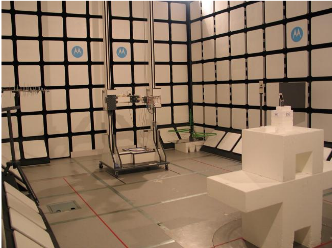
21616-1, IHDT56JM1 setup in semi-anechoic chamber – front view
