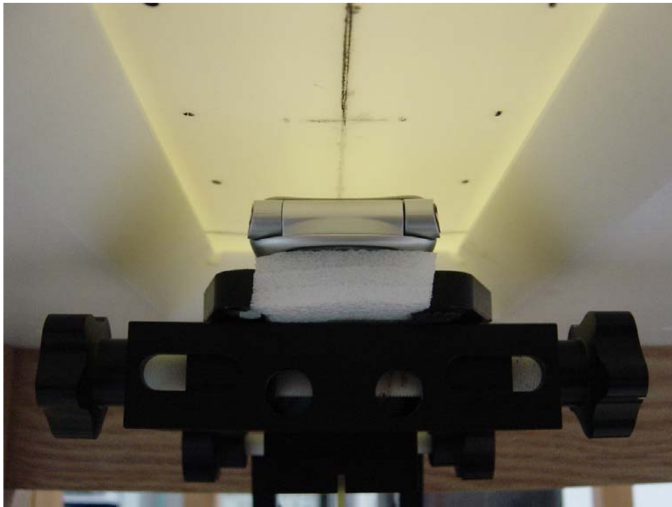
Figure 7: Phone Against the Flat Phantom
