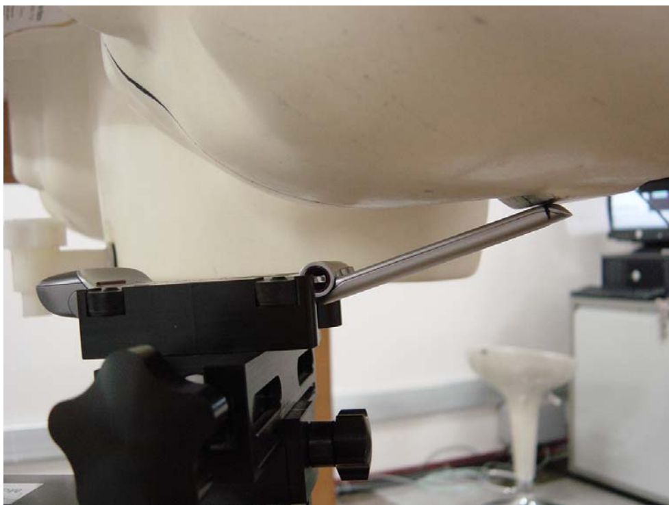
Figure 6: Phone Against the Head Phantom (15° Tilt)
