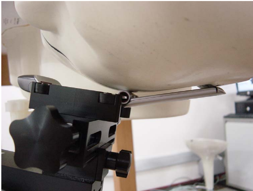
Figure 5: Phone Against the Head Phantom (Cheek Touch)
