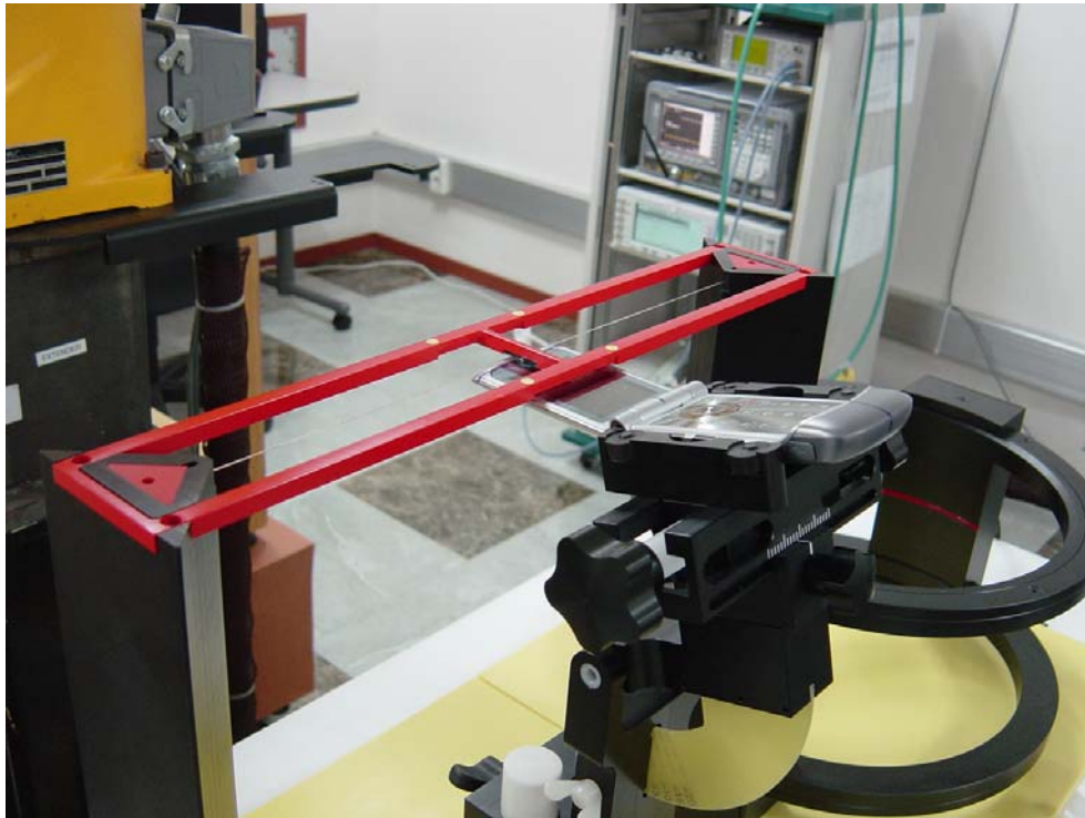
Figure A5-4. Positioning for RF Emissions
