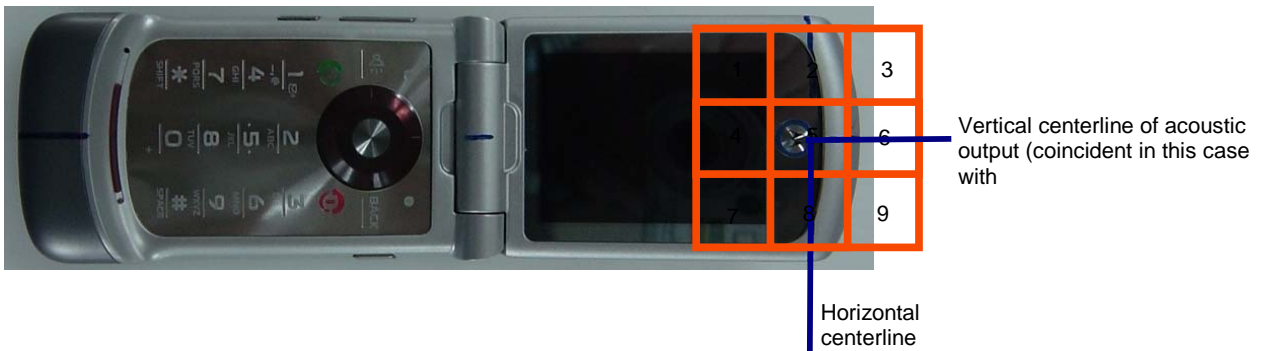
Figure A5-3. Phone Open - Orientation and Measurement Plane for RF Emissions Testing
