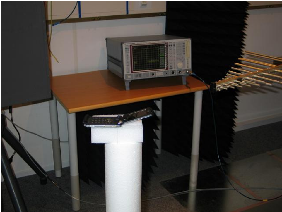
21620-1, IHDT56JJ1 check for maximum radiation at position X - Open
