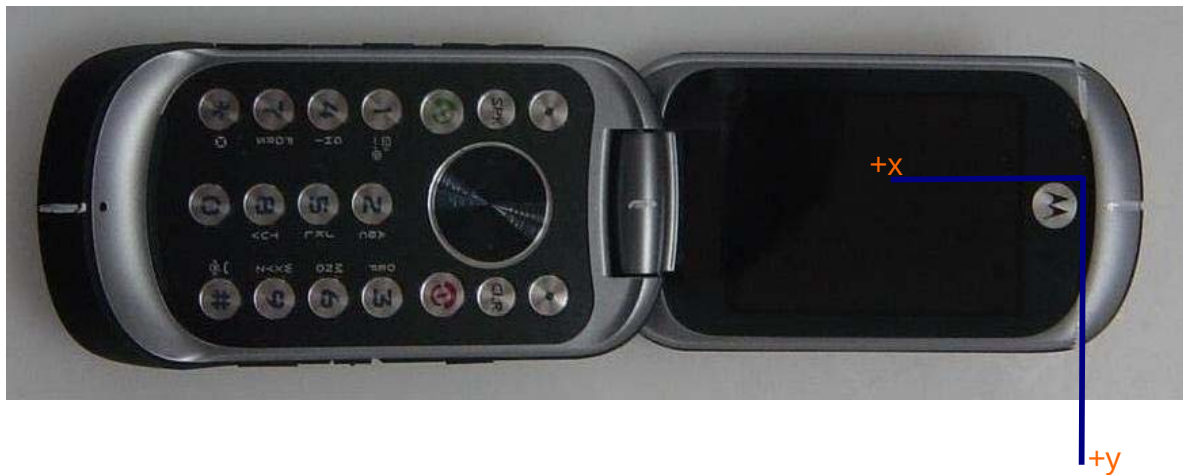
Figure A4-4. Coordinate Axis for T-coil Measurements
