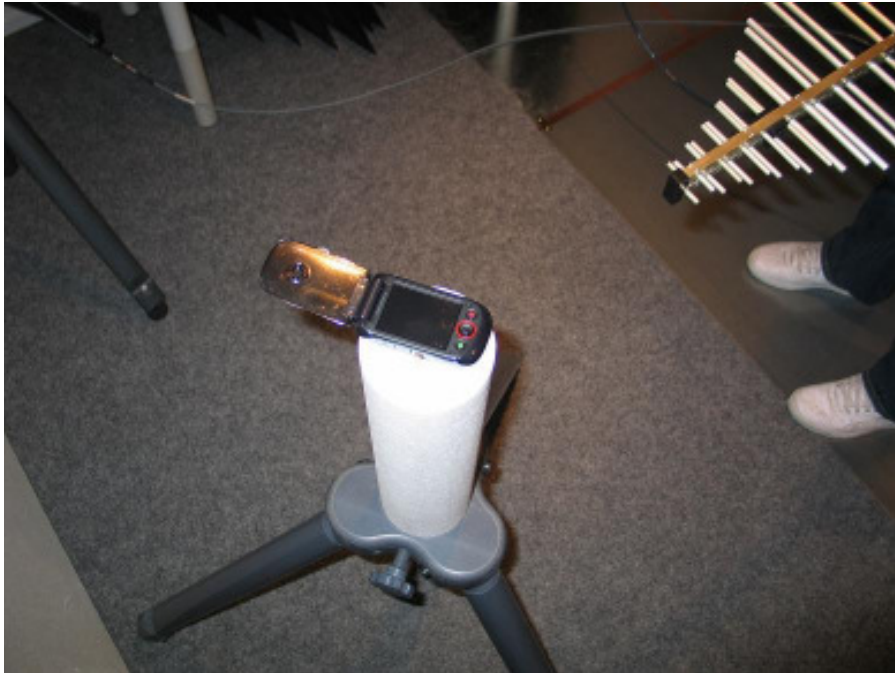
21699-1, IHDT56JF1 Check for maximum radiation at position X – Lid open
