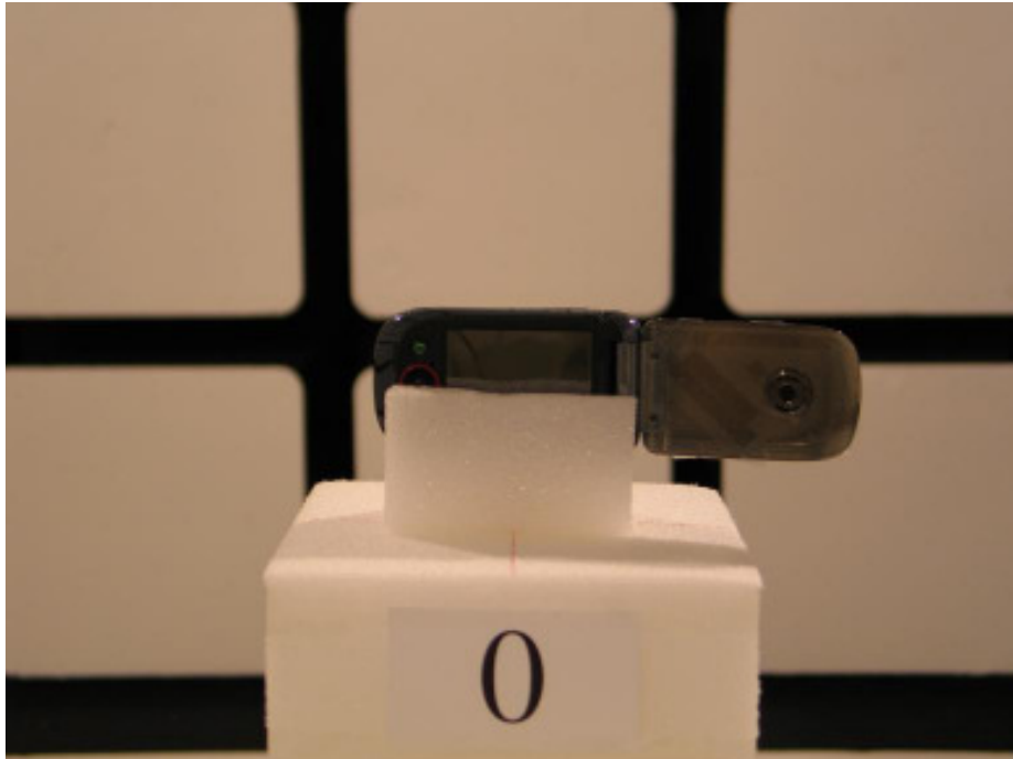
21699-1, IHDT56JF1 placed in test position Y – Lid open
