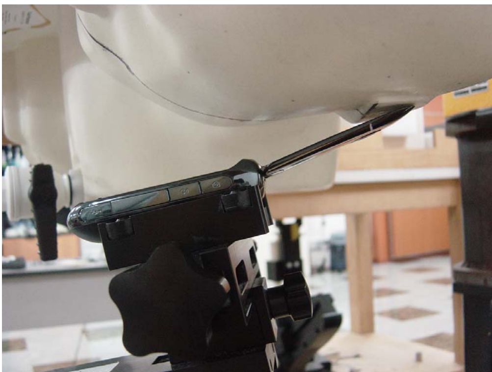
Figure 4: Phone Against the Head Phantom (15° Tilt)
