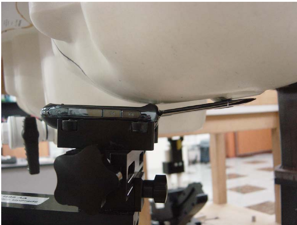
Figure 3: Phone Against the Head Phantom (Cheek Touch)
