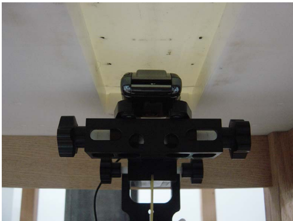
Figure 5: Phone Against the Flat Phantom
