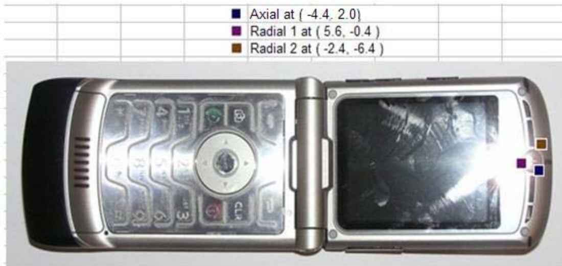
Figure A4-5. Location of Measured Points for T-coil measurements
