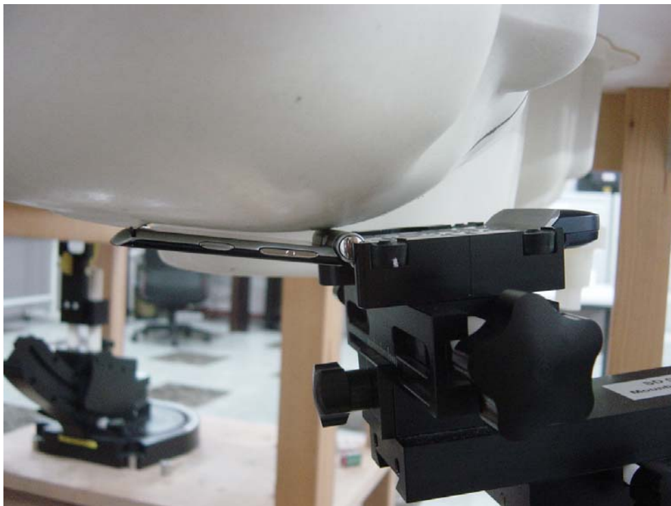
Figure 4: Phone Against the Head Phantom (Cheek Touch)
