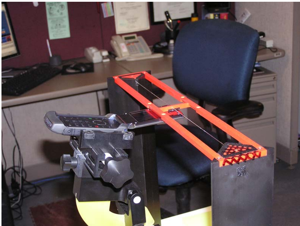
Figure A5-4. Positioning for RF Emissions
