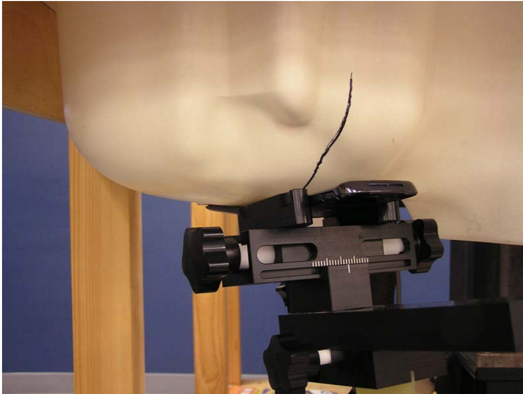
Figure 3 – Transceiver against head, Cheek Touch position
