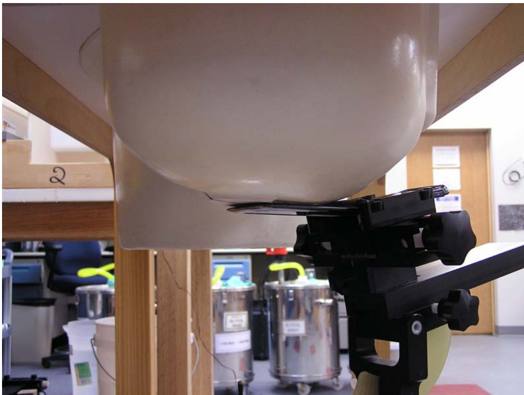
Figure 4 – Transceiver against head, Cheek Touch position
