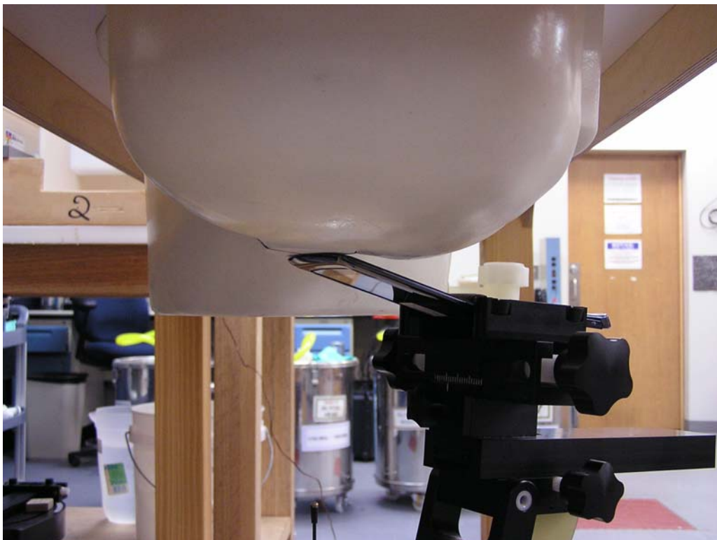
Figure 6 – Transceiver against head, 15° Tilt position
