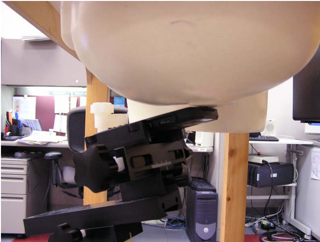
Figure 8 – Transceiver against head, 15° Tilt position
