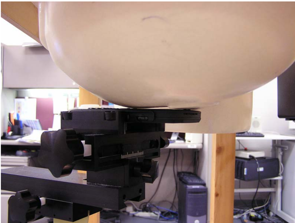
Figure 6 – Transceiver against head, Cheek Touch position
