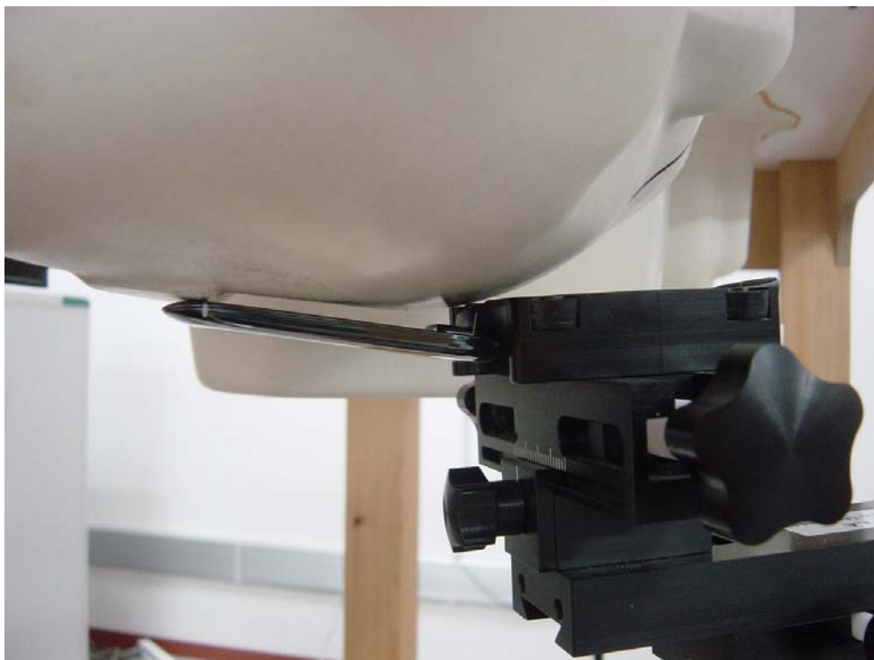
Figure 4. Phone Against the Head Phantom (Cheek Touch)
