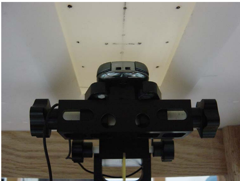
Figure 6. Phone Against the Flat Phantom
