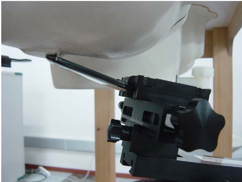
Figure 5. Phone Against the Head Phantom (15 degrees Tilt)
