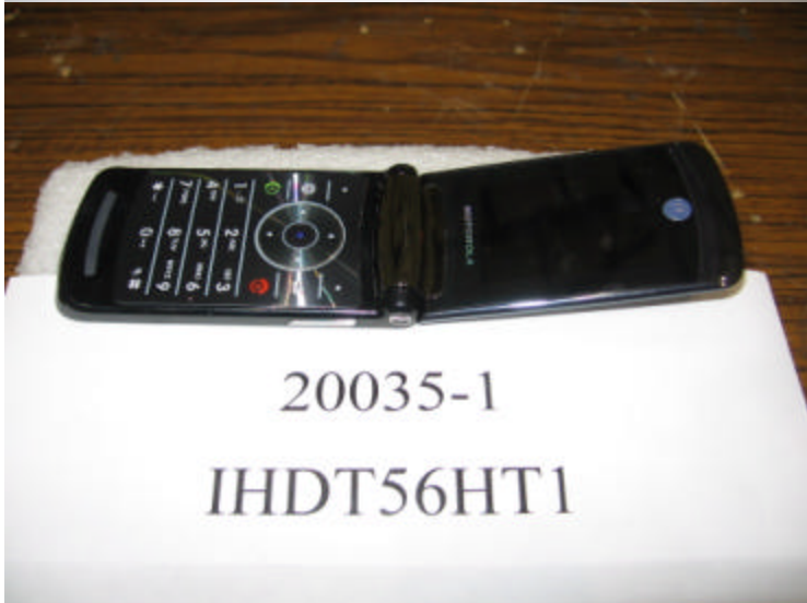
Radiated Emissions Z-Axis
