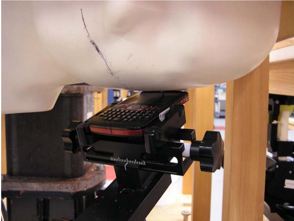
Figure 7 – Transceiver against head, 15° Tilt position
