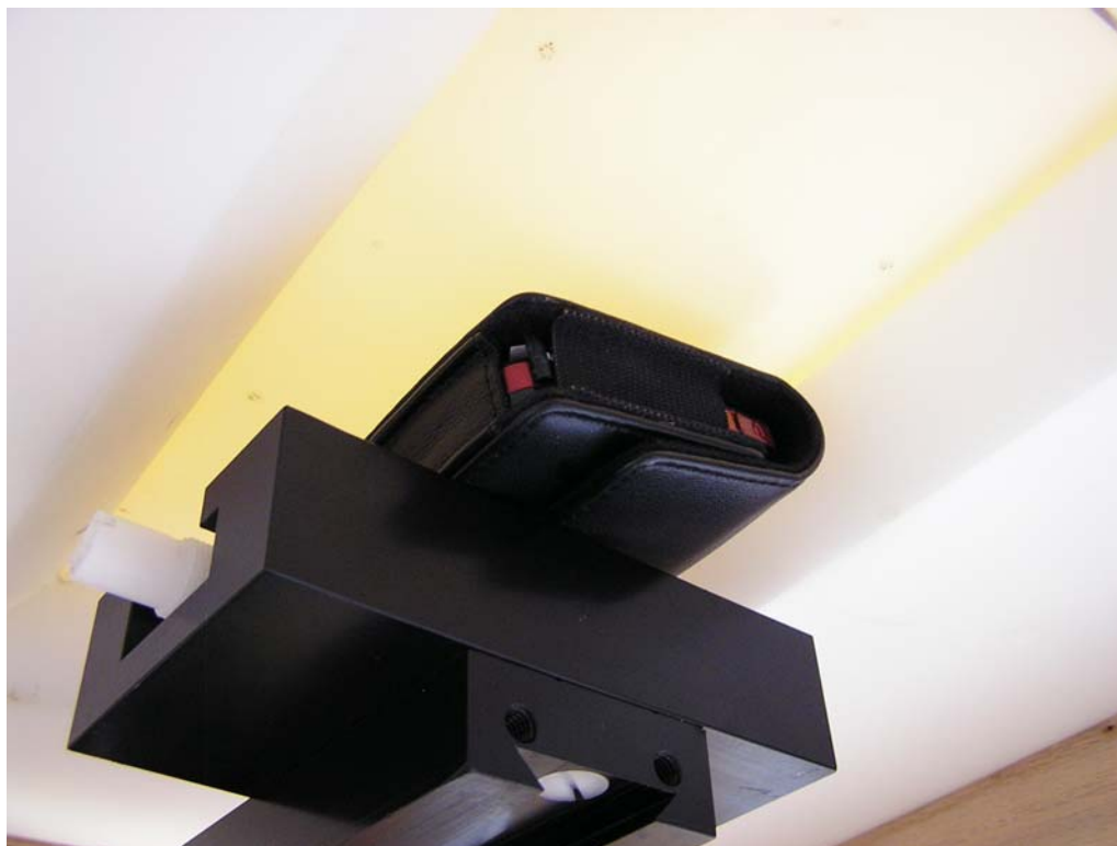
Figure 10 – Transceiver against body with Leather Pouch SYN1985A
