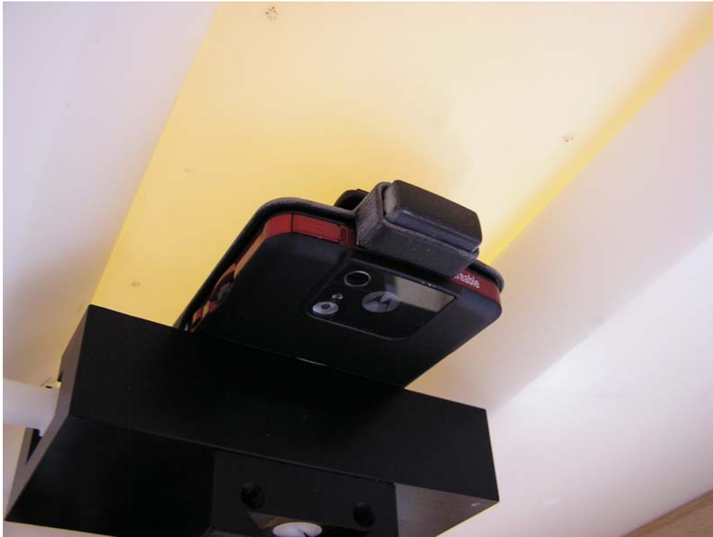
Figure 11 – Transceiver against body with Plastic Clip SYN2087A
