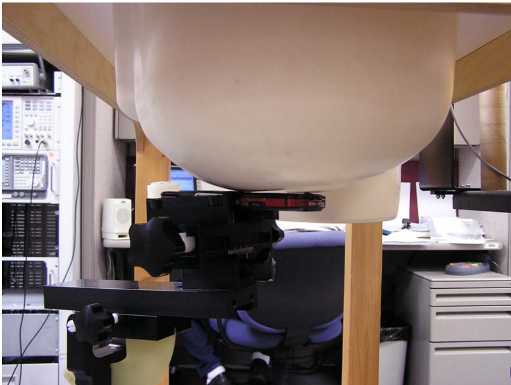
Figure 6 – Transceiver against head, Cheek Touch position
