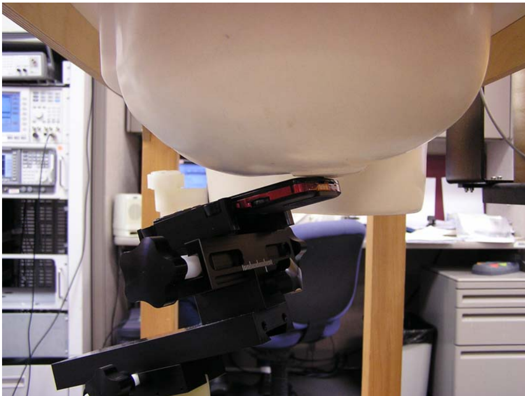
Figure 8 – Transceiver against head, 15° Tilt position
