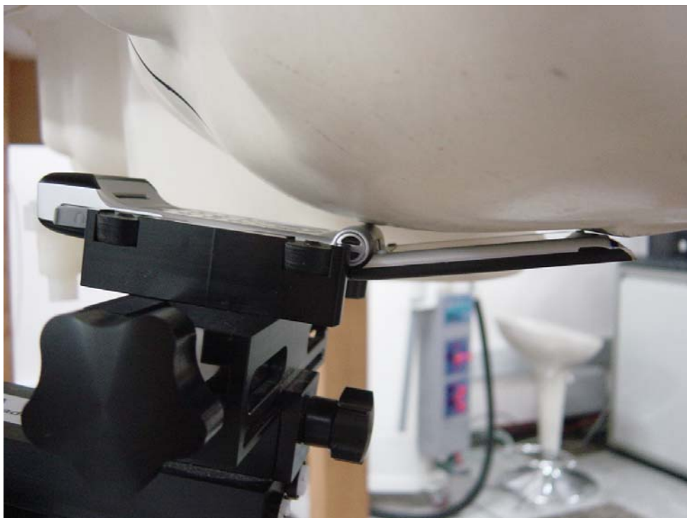
Figure 4. Phone Against the Head Phantom (Cheek Touch)
