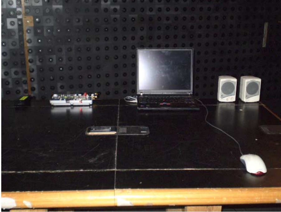
Photograph No.9 Unintentional radiated emission measurements setup EUT close view
