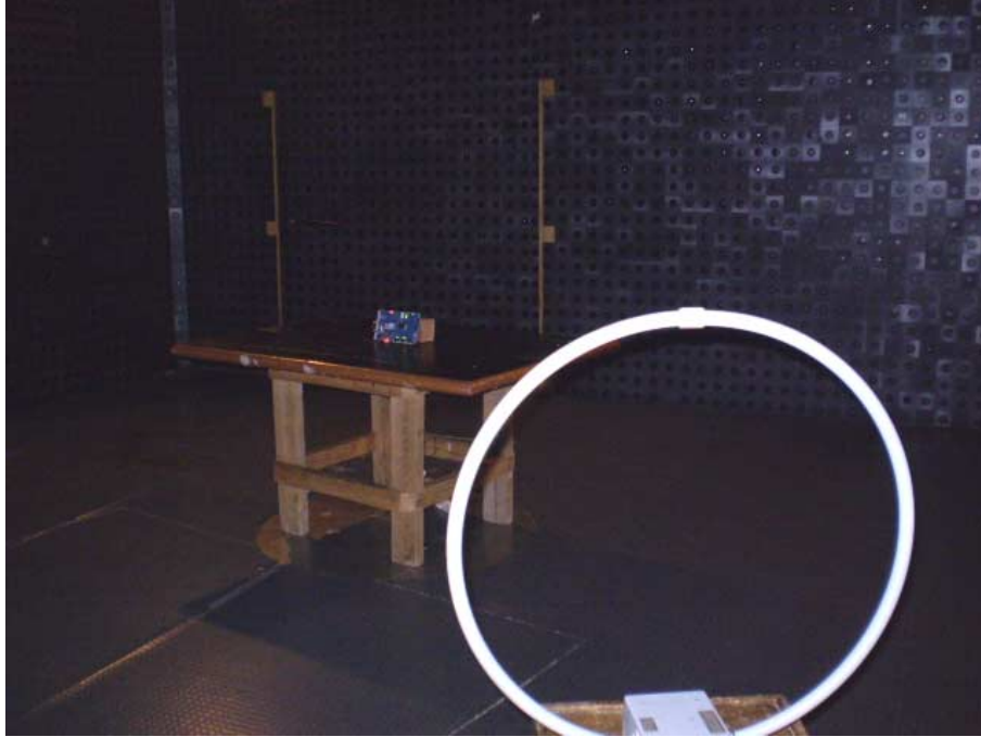
Photograph No.4 Radiated emissions measurement setup in the anechoic chamber with loop antenna
