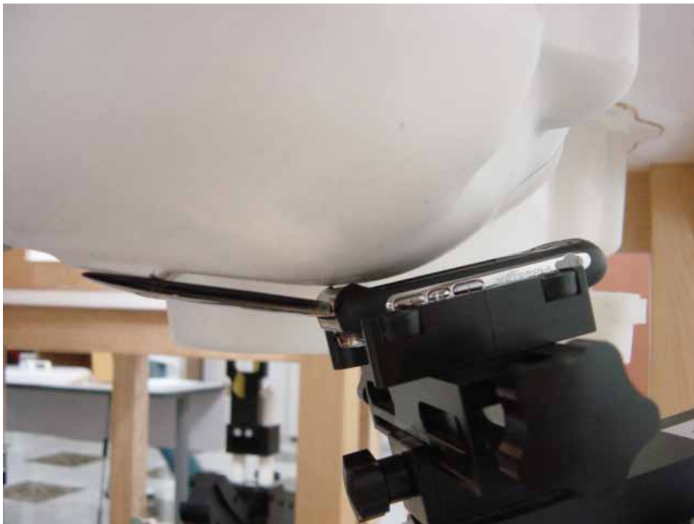
Figure5: Phone Against the Head Phantom (Cheek Touch)
