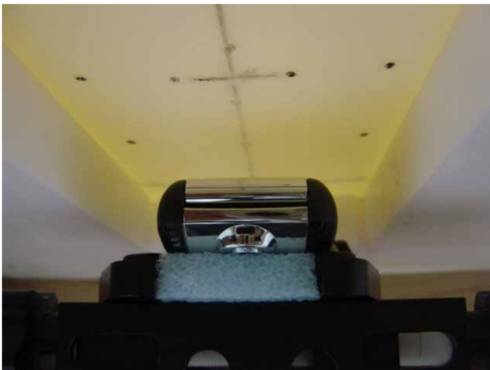
Figure4: Phone Against the Flat Phantom
