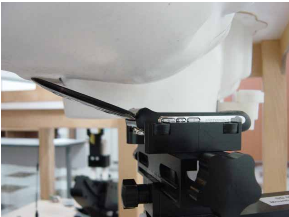
Figure6: Phone Against the Head Phantom (15° Tilt)
