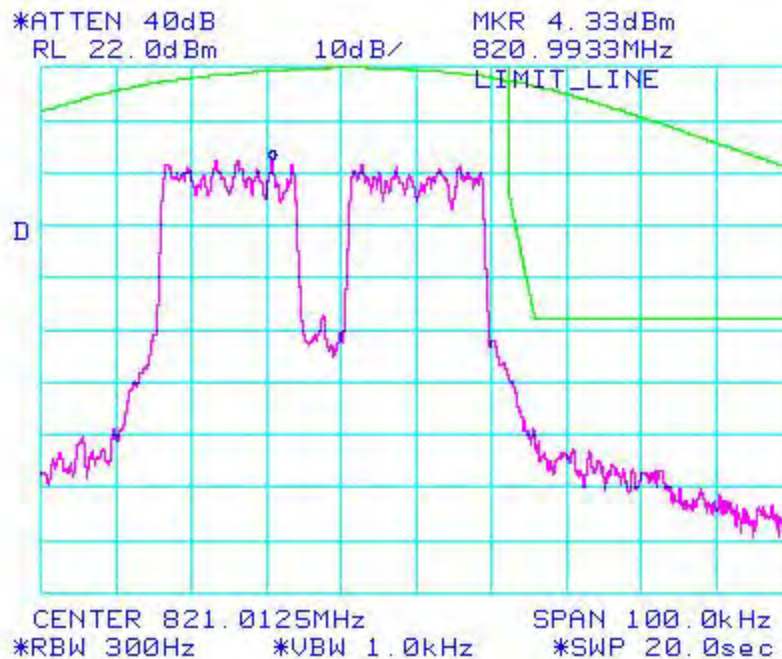
Figure 6a-2.4.5. WiDEN50 800 MHz Band, Continuous QAM64, Maximum Power, EA Emission Mask
