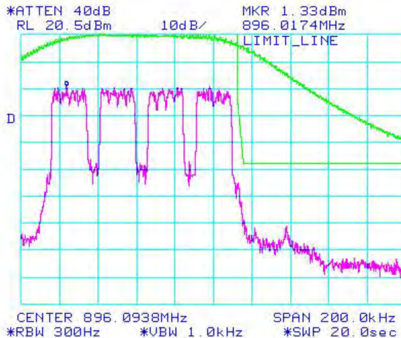
Figure 6a-2.11.3. WiDEN100 900 MHz Band, QAM16, Maximum Power, EA Emission Mask
