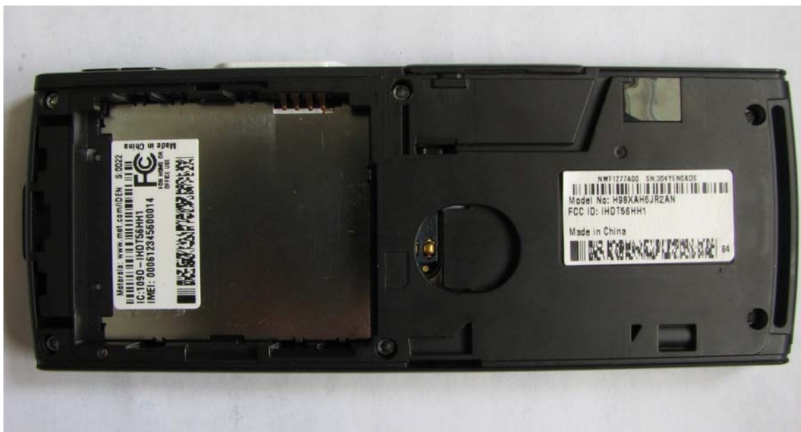
Figure 3-7. Battery Compartment of i425 radio.
