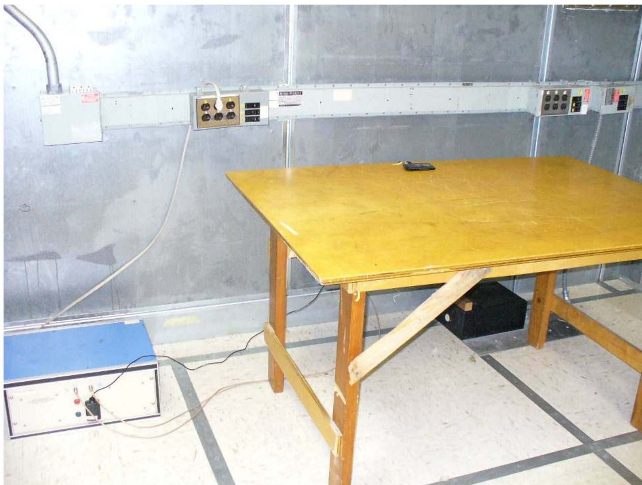
Figure 1: UUT connected to Rapid Rate Charger.
