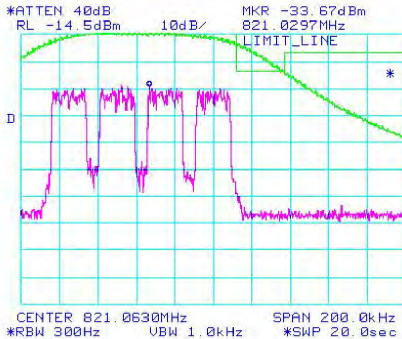
Figure 6a-2.6.4. WiDEN100 800 MHz Band, QAM16, Minimum Power, EA Emission Mask
