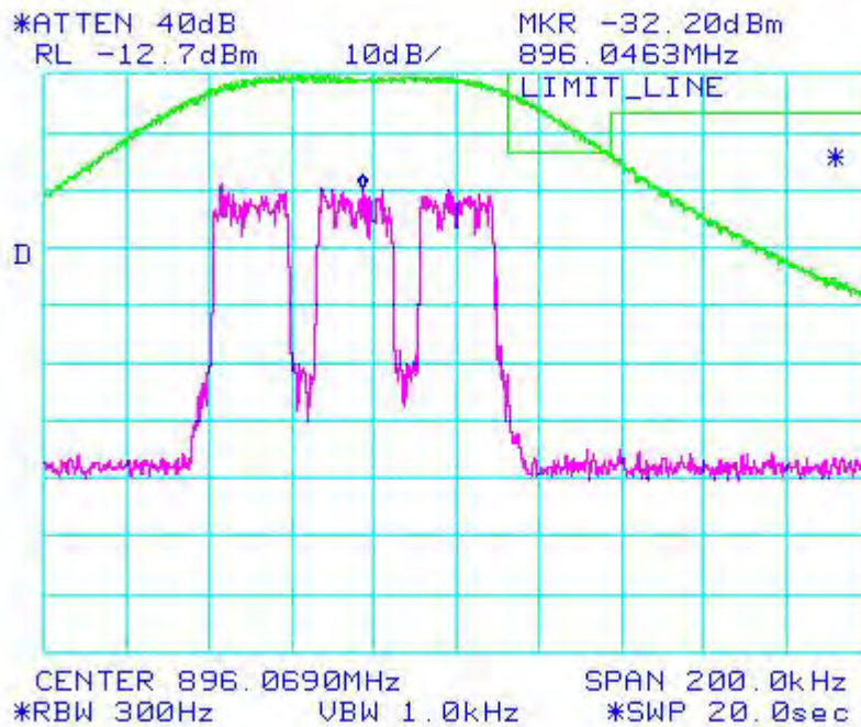
Figure 6a-2.10.6. WiDEN75 900 MHz Band, QAM64, Minimum Power, EA Emission Mask
