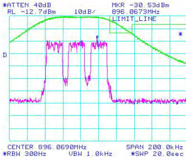
Figure 6a-2.10.4. WiDEN75 900 MHz Band, QAM16, Minimum Power, EA Emission Mask
