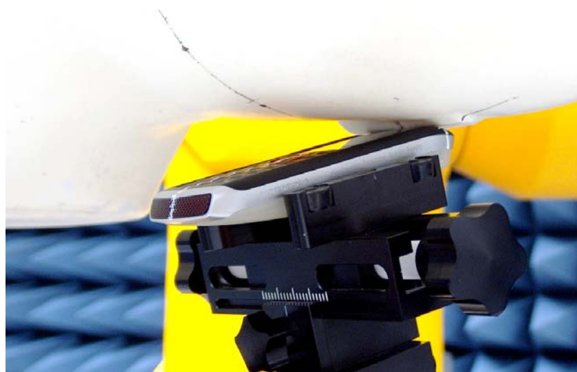
Figure 7: Assessment at the Head DUT at the left ear in tilt position
