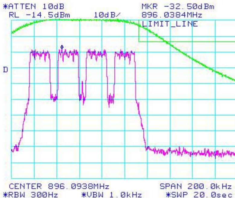
Figure 6a-2.11.4. WiDEN100 900 MHz Band, QAM16, Minimum Power, EA Emission Mask
