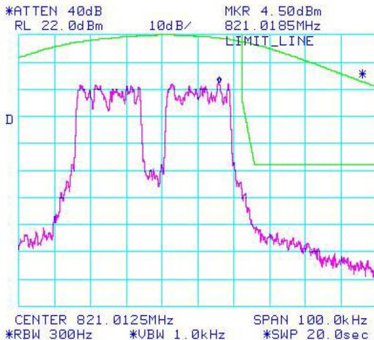
Figure 6a-2.4.1. WiDEN50 800 MHz Band, Continuous Quad-QPSK, Maximum Power, EA Emission Mask
