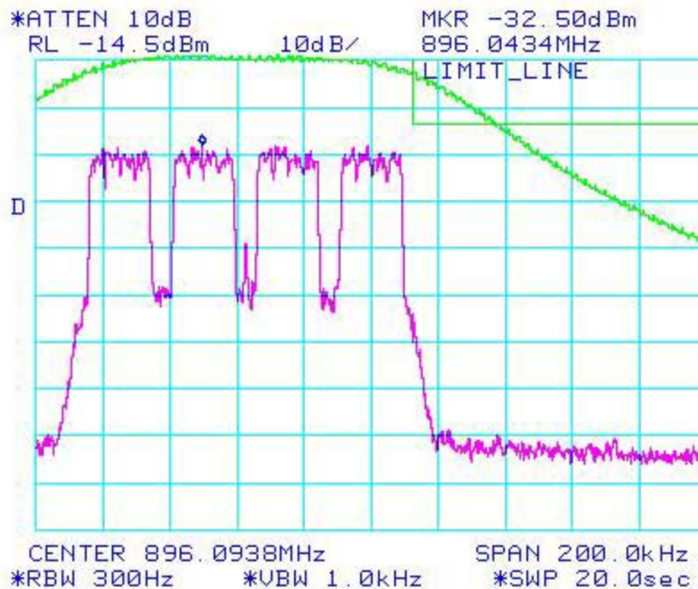
Figure 6a-2.11.6. WiDEN100 900 MHz Band, QAM64, Minimum Power, EA Emission Mask
