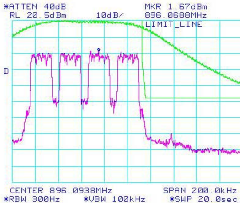
Figure 6a-2.11.5. WiDEN100 900 MHz Band, QAM64, Maximum Power, EA Emission Mask
