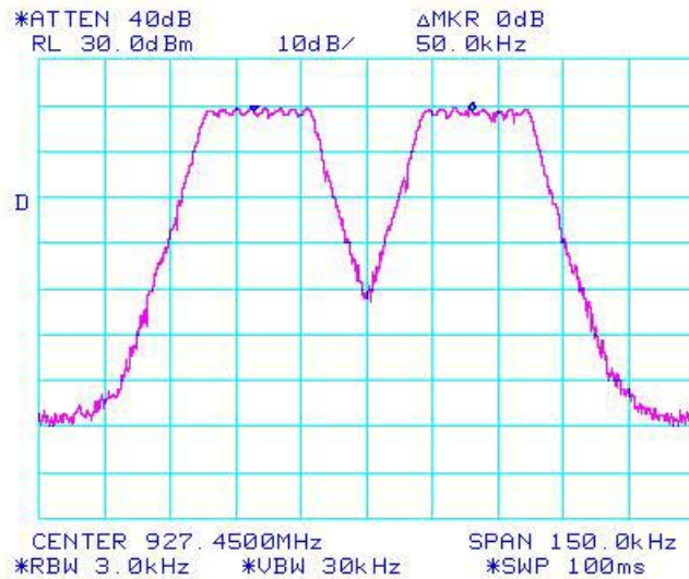
Figure 6c.2.2.6. Adjacent hop set separation with spectrum analyzer center frequency 927.5 MHz.
