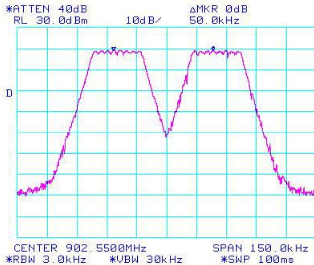
Figure 6c.2.2.2. Adjacent hop set separation with spectrum analyzer center frequency at 902.55 MHz.
